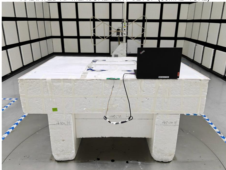
RADIATED RF MEASUREMENT SETUP (Below 30MHz)
