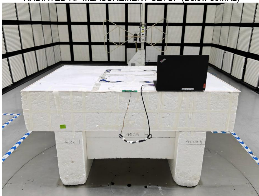
RADIATED RF MEASUREMENT SETUP (Below 30MHz)
