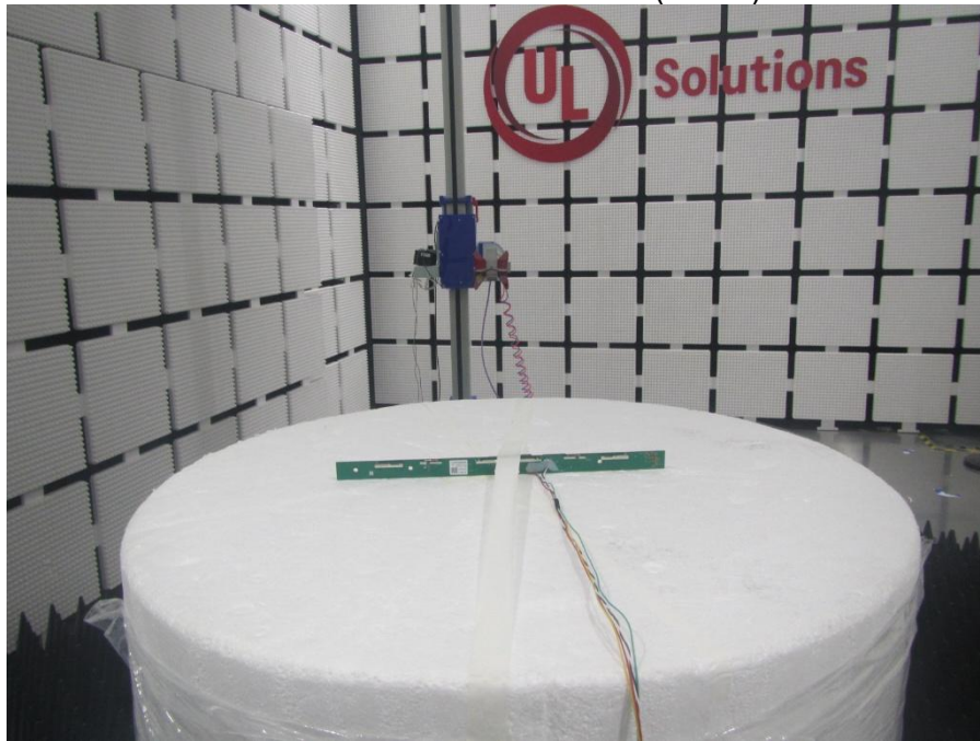
RADIATED RF MEASUREMENT SETUP (30MHz~1GHz)
