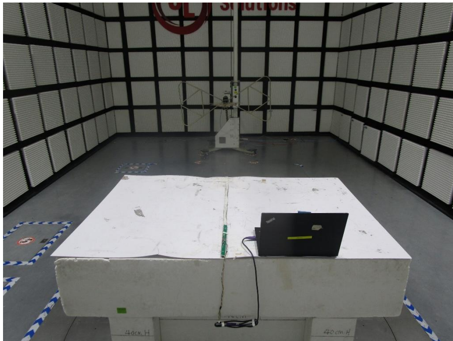
RADIATED RF MEASUREMENT SETUP (30MHz~1GHz)
