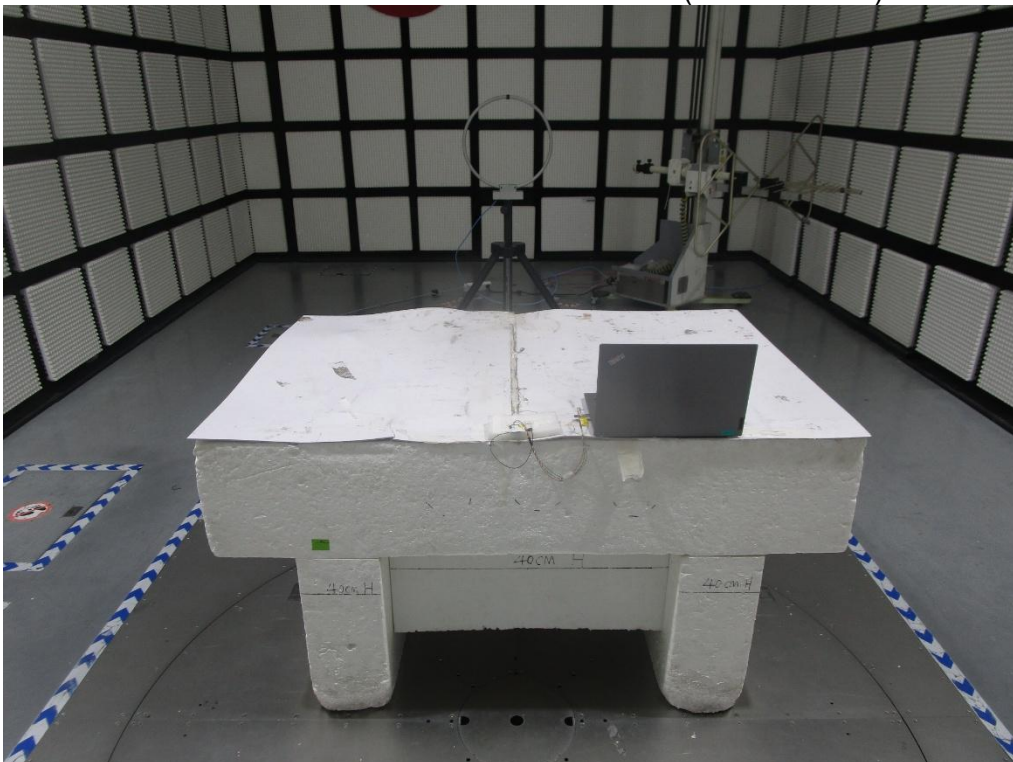
RADIATED RF MEASUREMENT SETUP (Below 30MHz)
