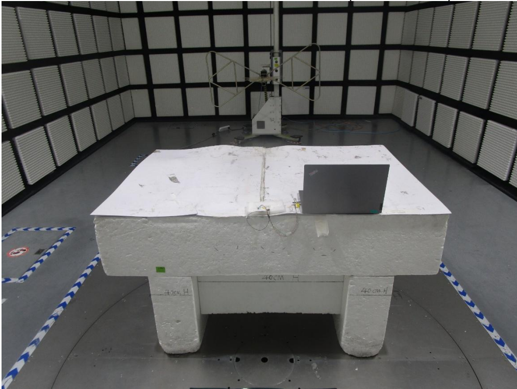
RADIATED RF MEASUREMENT SETUP (Below 30MHz)
