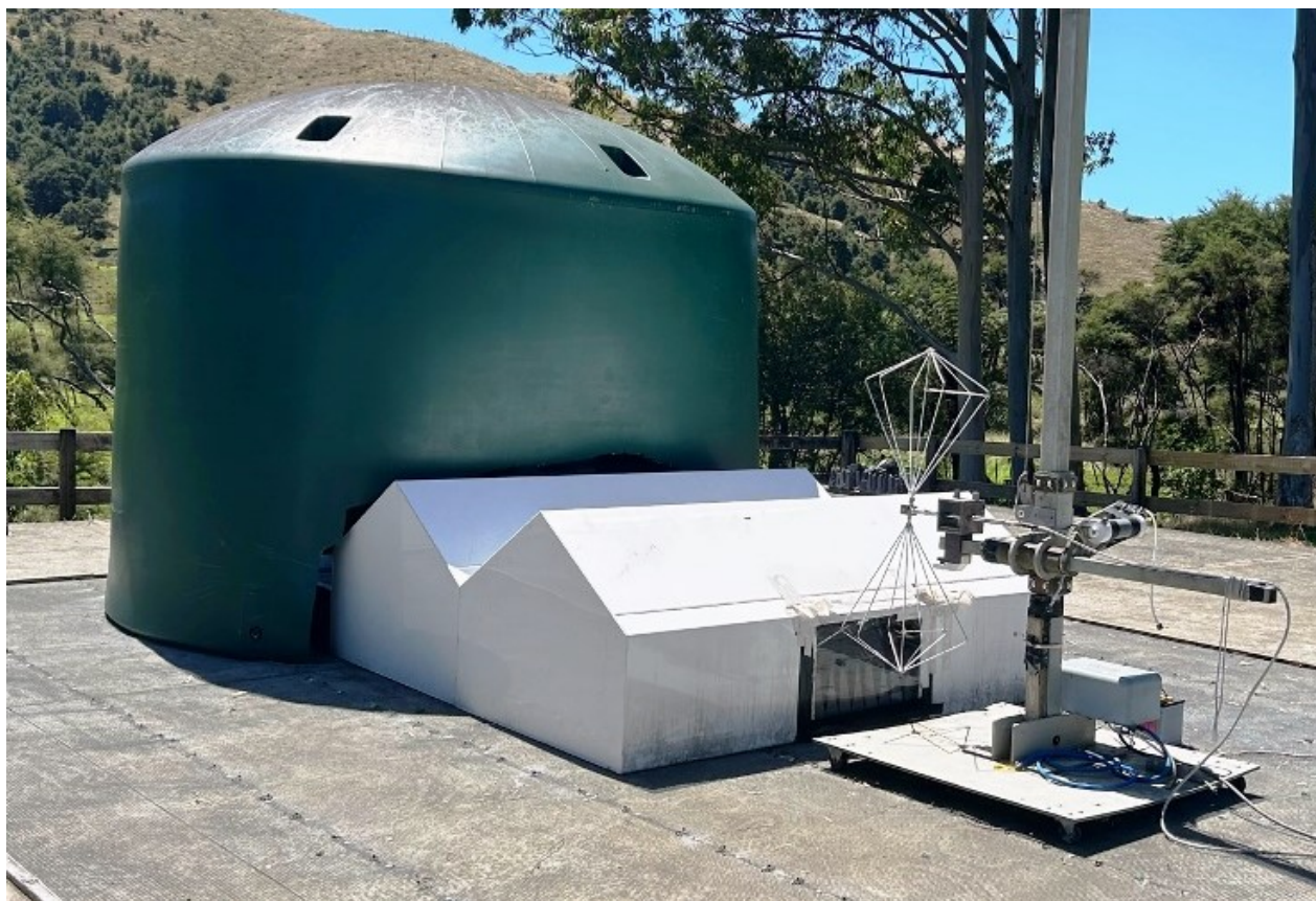
Log Periodic Antenna pointing towards Test Shed
