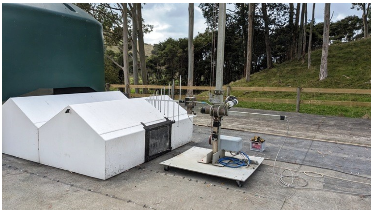
Log Periodic Antenna pointing towards Test Shed
