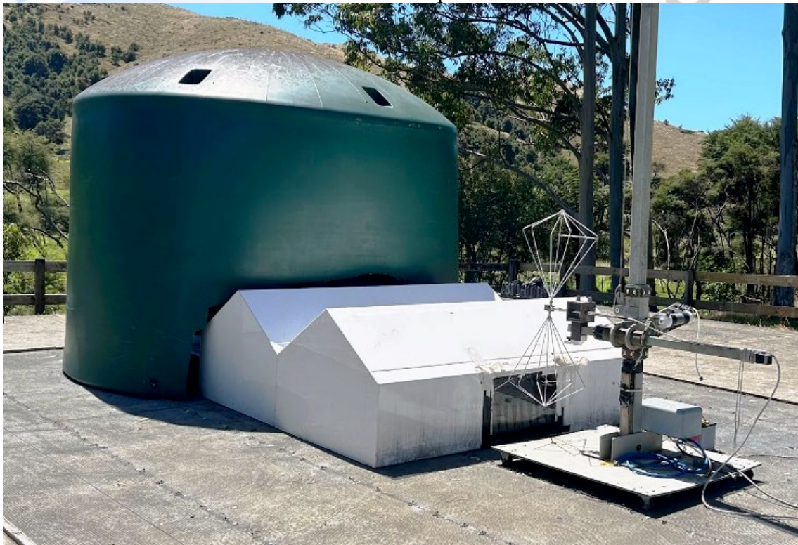
Radiated Emissions Test Setup - Biconical Antenna
