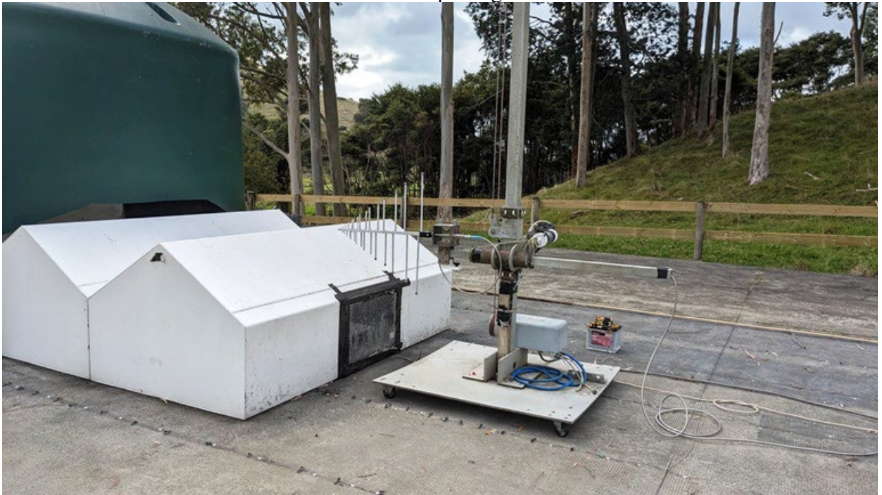
Radiated Emissions Test Setup - Horn Antenna
