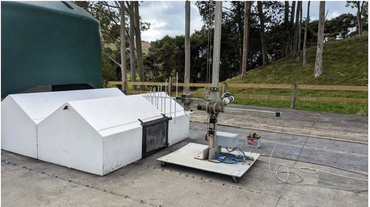
Radiated Emissions Test Setup - Log Periodic Antenna
