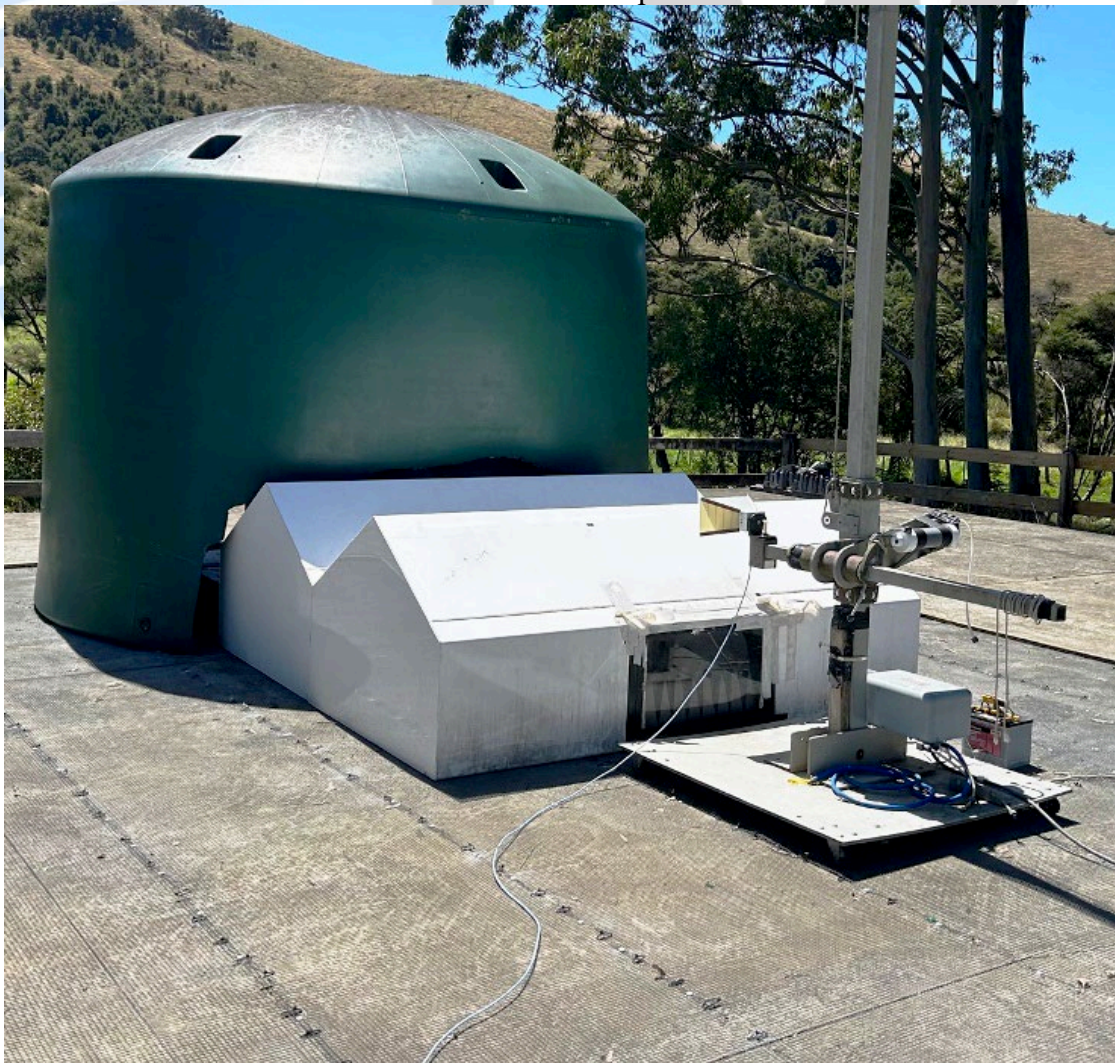
Radiated Emissions Test Setup - Horn Antenna
