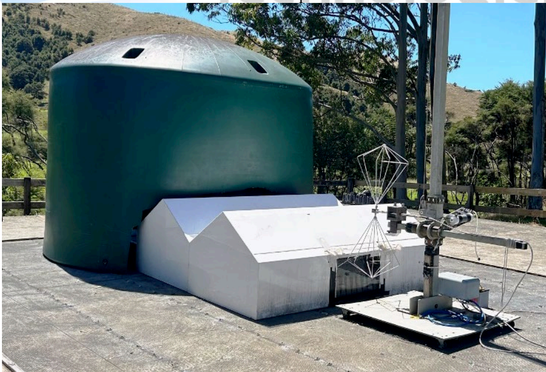
Radiated Emissions Test Setup - Biconical Antenna
