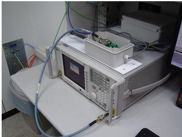
Photo 1. RF conducted emission test.
