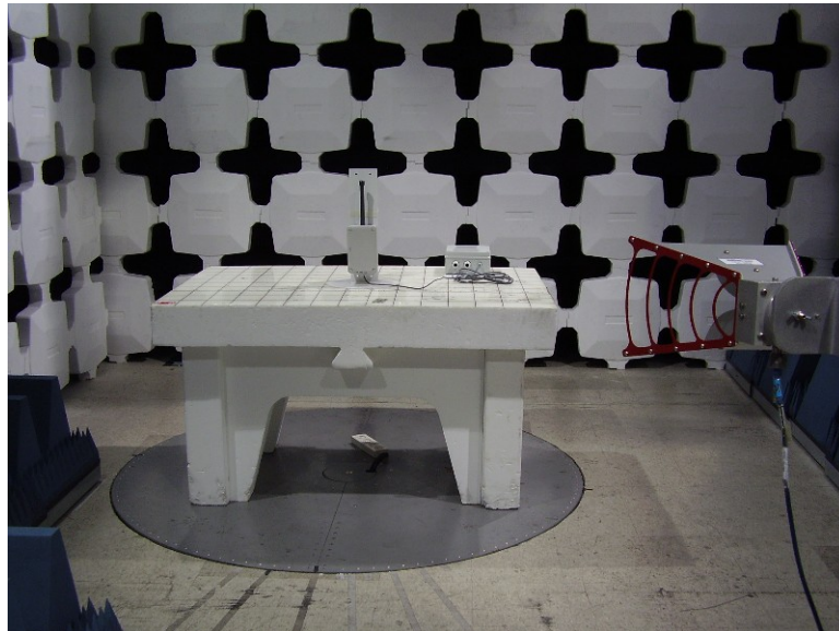
Photo 3. Radiated emissions test.
