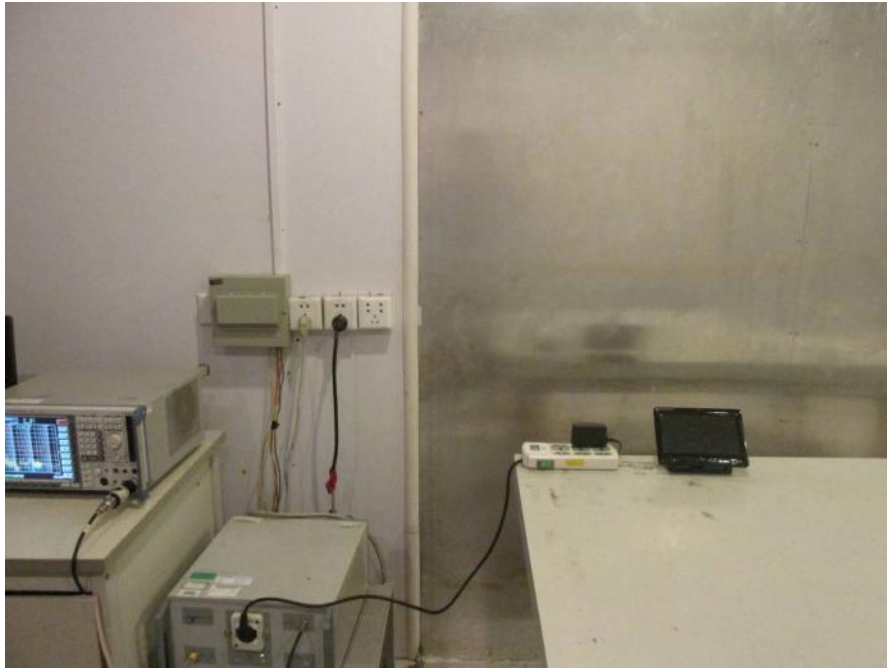
CONDUCTED EMISSION TEST
