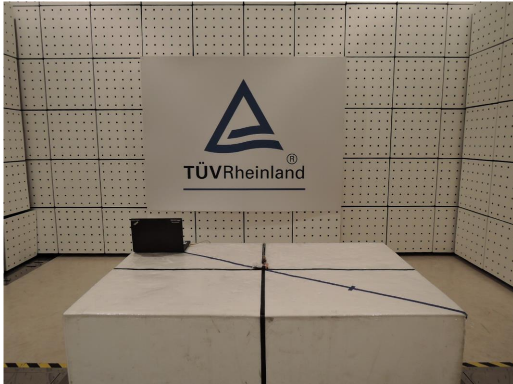
Photograph 1: Set-up for Spurious Emissions (Front View)
