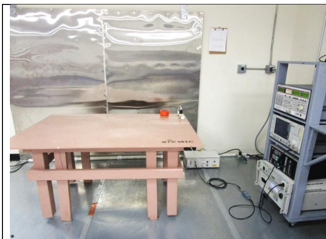
AC Line Conducted Emissions – Front View
