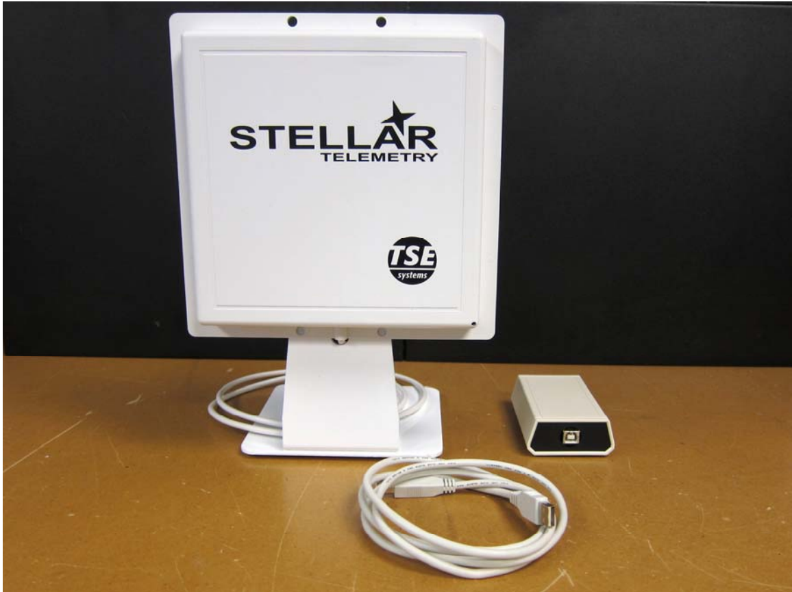
Antenna Cable and Transmitter
