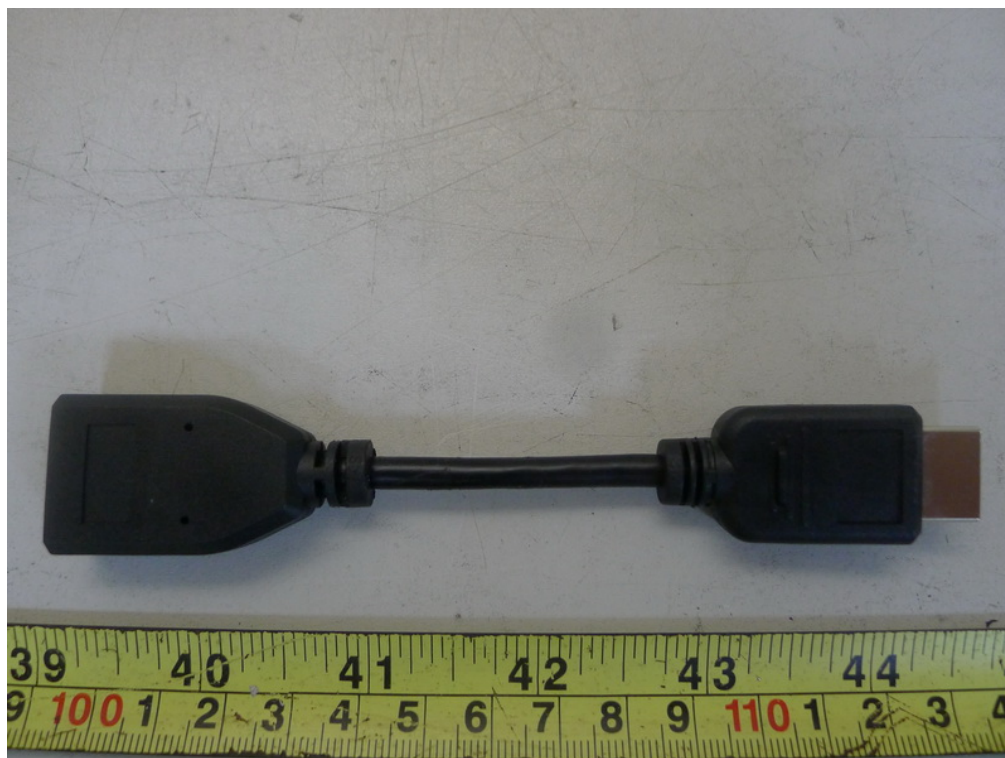
HDMI Extension Cable (BMS)
