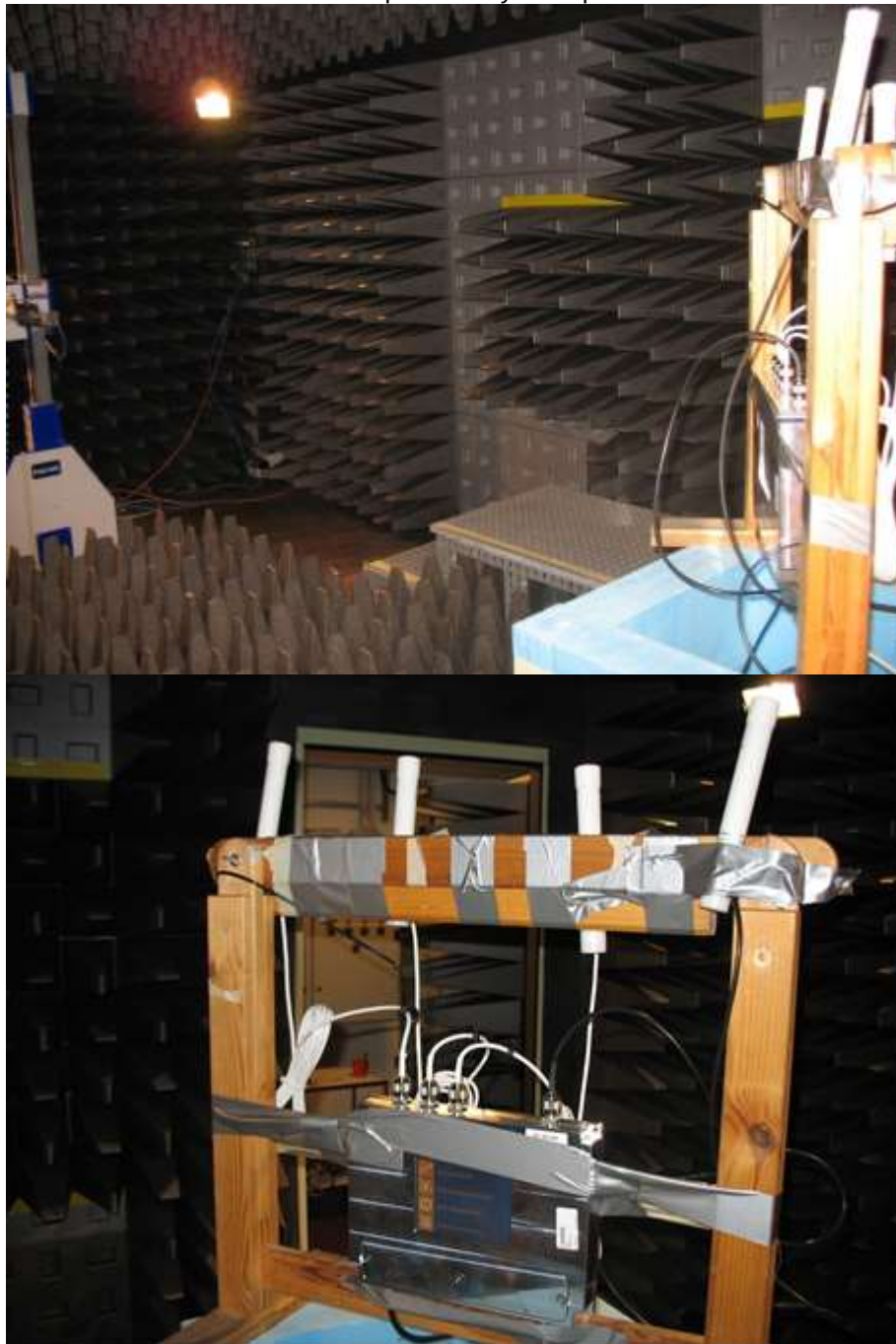
Radiated emission 18 – 40 GHz preliminary sweep
