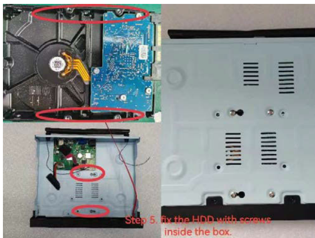
Step 5. fix the HDD with screws inside the box.
