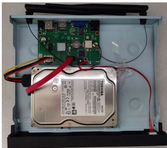
Step 4. Mount the HDD to the DVR/NVR system match the 4 connections holes.
