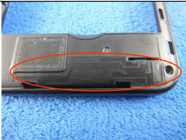
GSM/PCS/UMTS-FDD Antenna View
