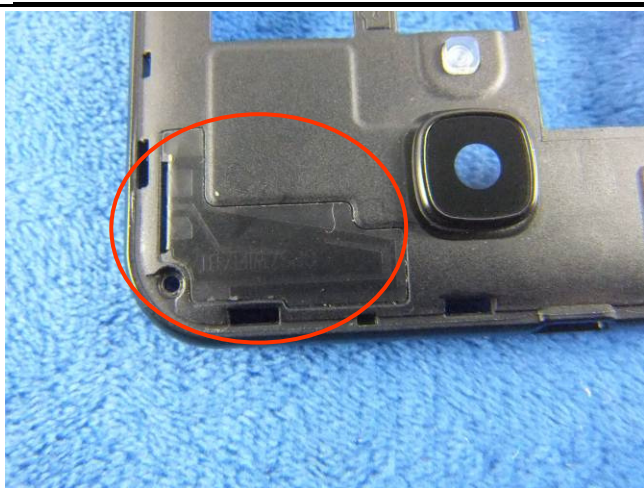
WIFI/BT/BLE/GPS - Antenna View
