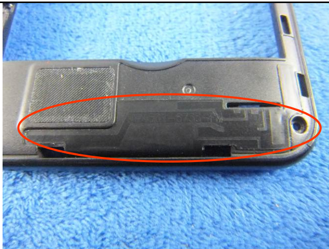
GSM/PCS/UMTS-FDD Antenna View
