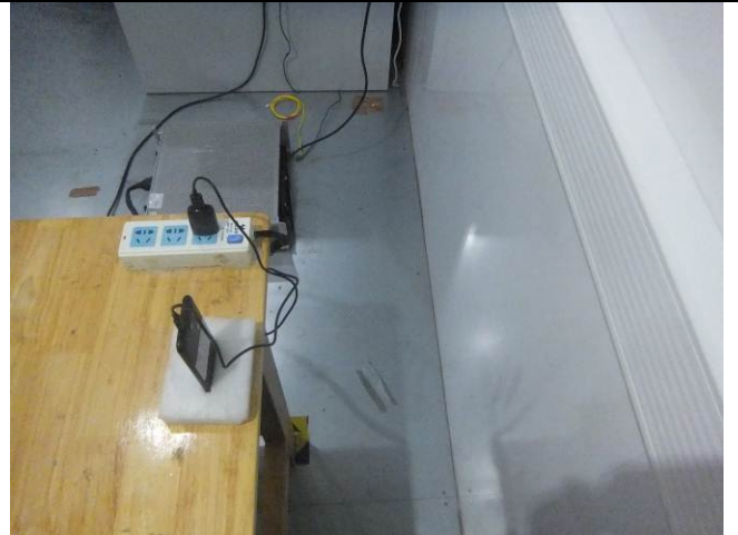
Conducted Emissions Test Setup Side View
