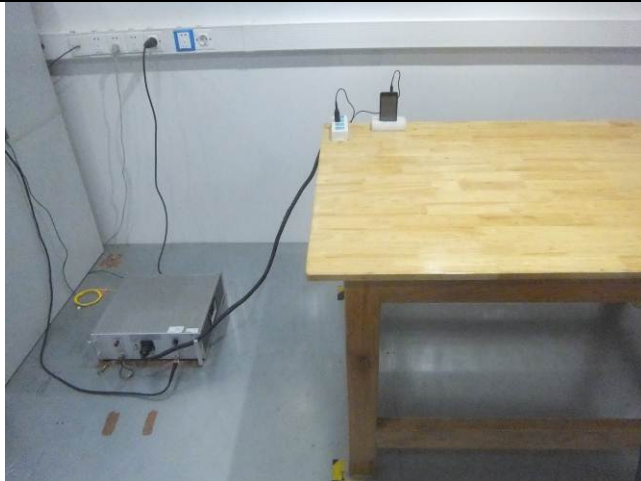
Conducted Emissions Test Setup Front View
