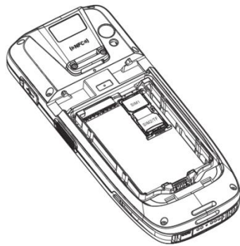
Figure 4-2 Insert the SIM Card
