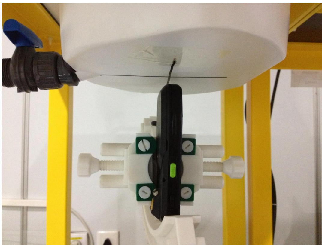
Fig.10 Body Edge C(Down,10mm separation)
