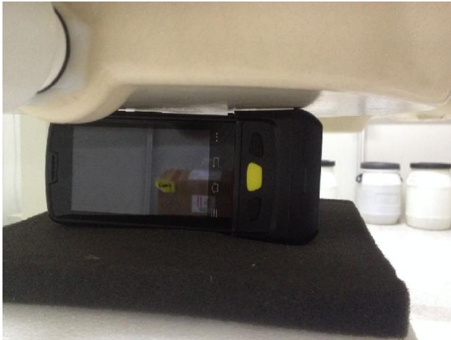
Body SAR Right Side 0mm for GSM/UMTS
