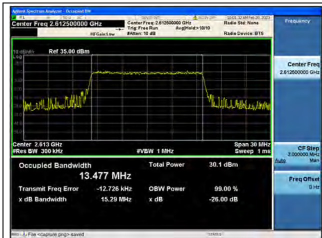
Band38 / 15MHz / QPSK/ High CH
