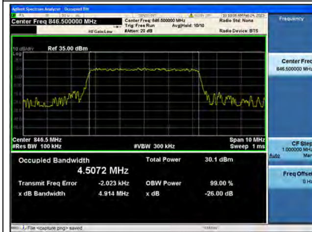
Band5 / 5MHz / 64QAM/ High CH
