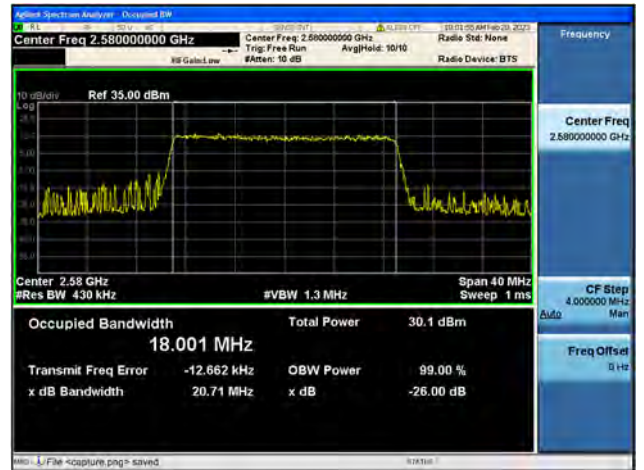
Band38 / 20MHz / QPSK/ Low CH
