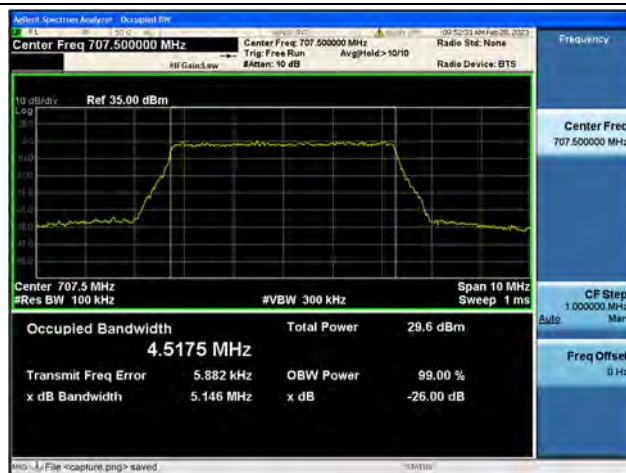
Band12 / 5MHz / 16QAM/ Mid CH
