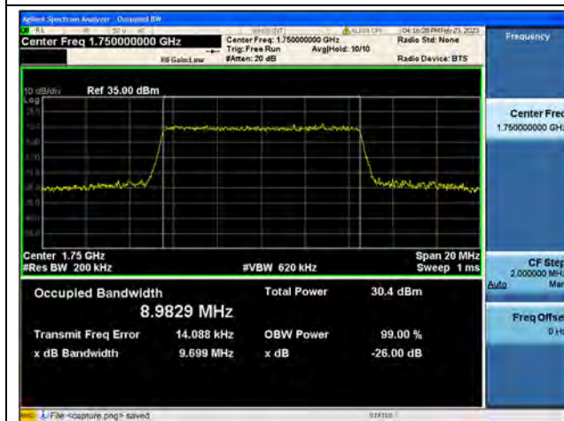
Band4 / 10MHz / 16QAM/ High CH
