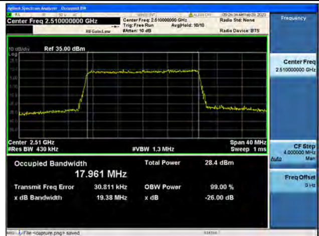
Band7 / 20MHz / 64QAM/ Low CH
