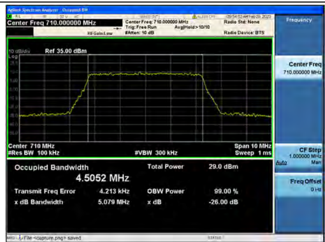
Band17 / 5MHz / 64QAM/ Mid CH
