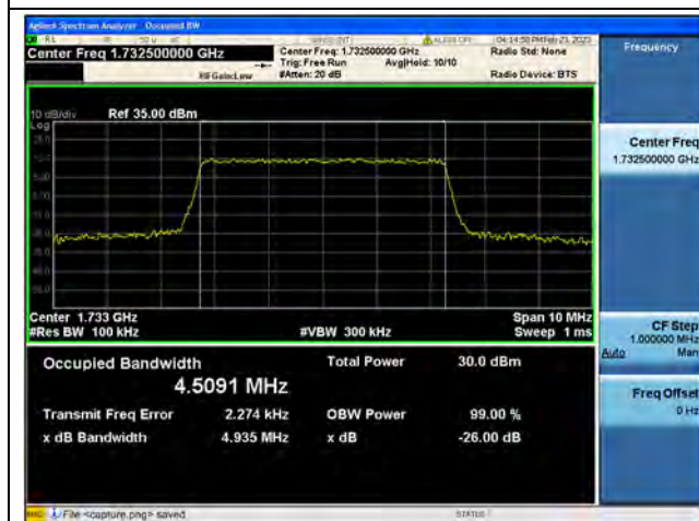
Band4 / 5MHz / 16QAM/ Mid CH
