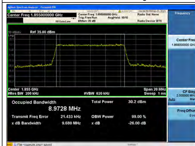
Band2 / 10MHz / 16QAM/ Low CH
