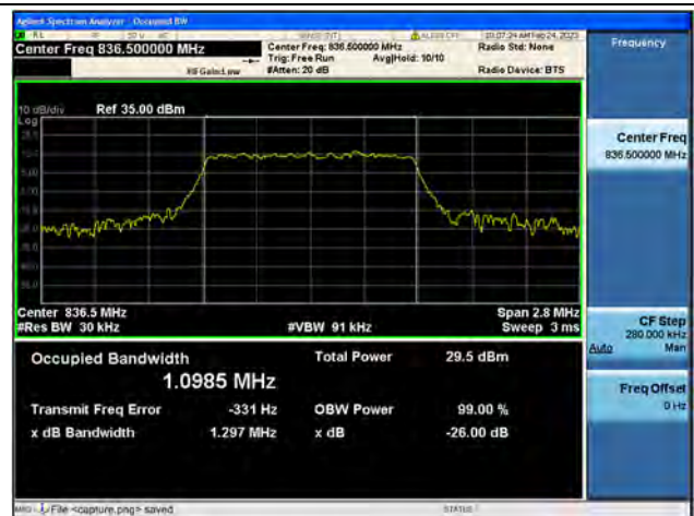
Band5 / 1.4MHz / 64QAM/ Mid CH
