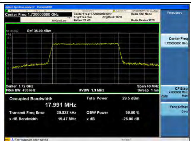
Band4 / 20MHz / 64QAM/ Low CH
