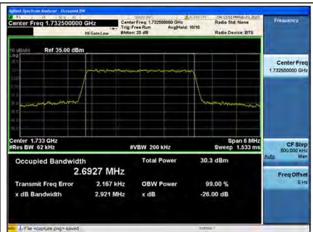
Band4 / 3MHz / 16QAM/ Mid CH
