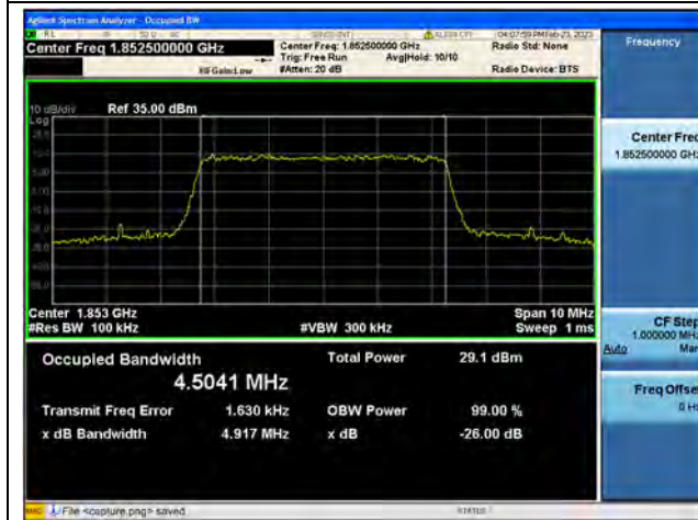
Band2 / 5MHz / 64QAM/ Low CH
