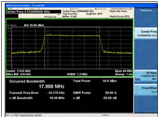
Band7 / 20MHz / QPSK/ Mid CH
