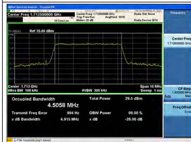
Band4 / 5MHz / 64QAM/ Low CH
