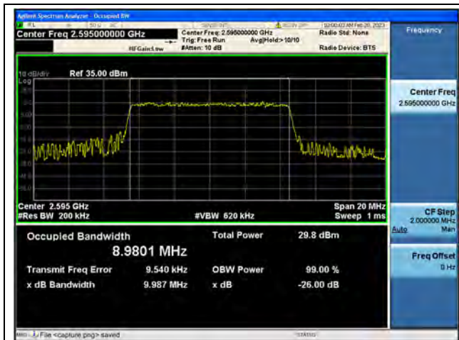
Band38 / 10MHz / QPSK/ Mid CH
