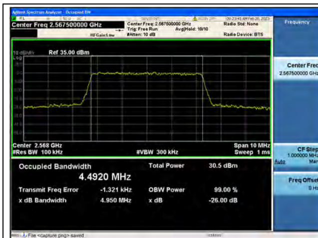
Band7 / 5MHz / QPSK/ High CH
