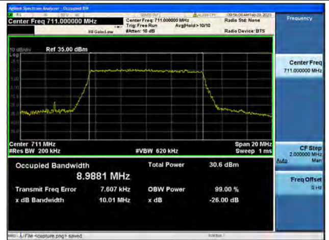
Band17 / 10MHz / QPSK/ High CH
