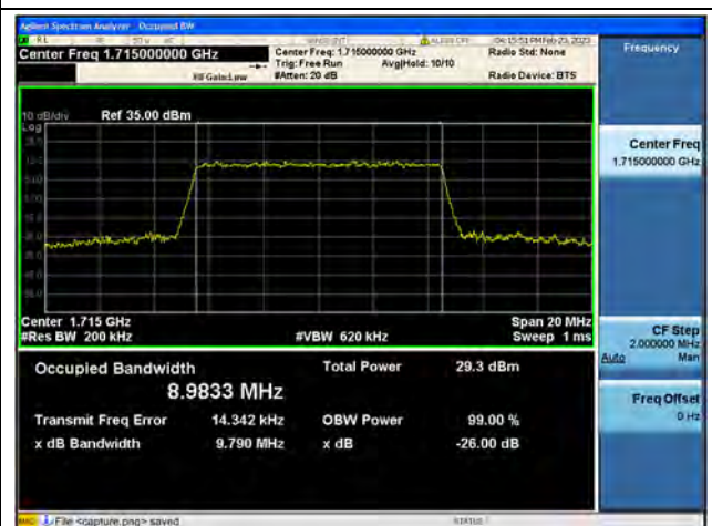
Band4 / 10MHz / 64QAM/ Low CH
