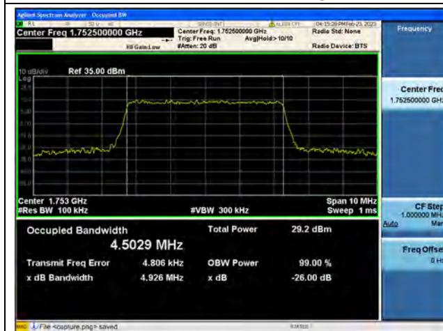
Band4 / 5MHz / 64QAM/ High CH
