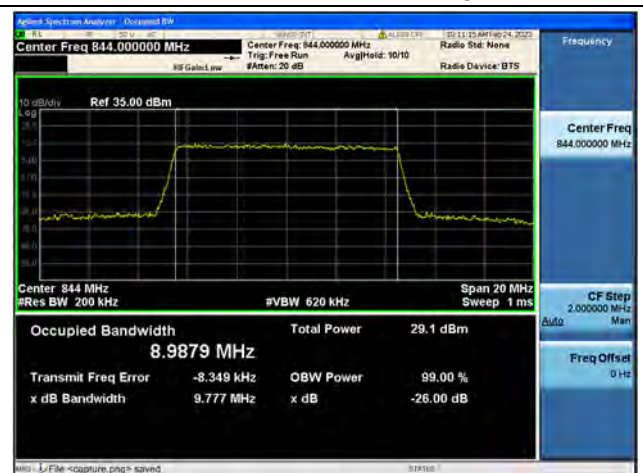
Band5 / 10MHz / 64QAM/ High CH
