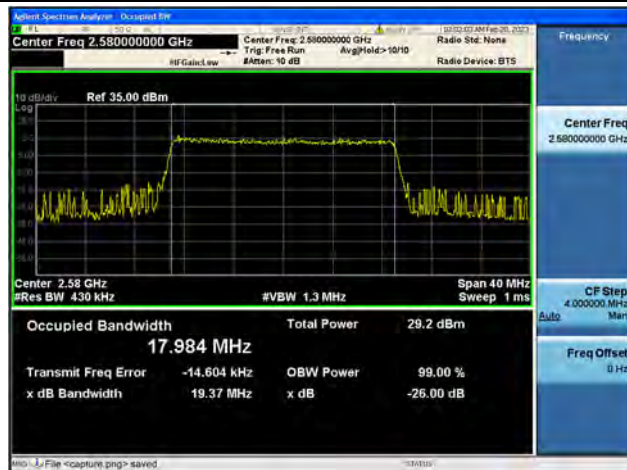
Band38 / 20MHz / 16QAM/ Low CH
