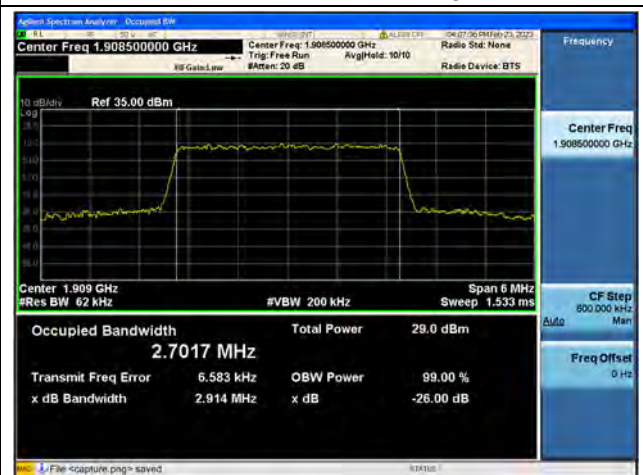
Band2 / 3MHz / 64QAM/ High CH
