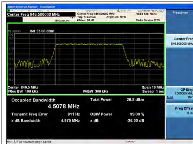
Band5 / 5MHz / QPSK/ High CH
