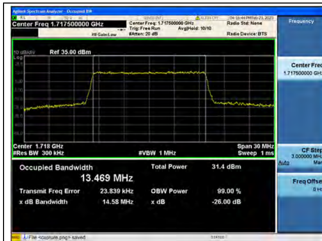
Band4 / 15MHz / QPSK/ Low CH
