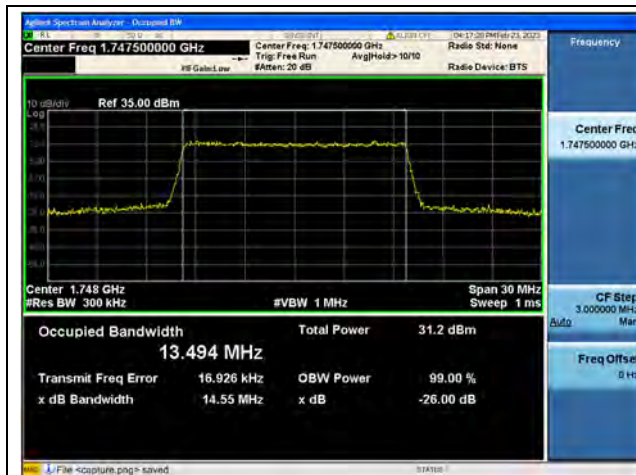
Band4 / 15MHz / QPSK/ High CH
