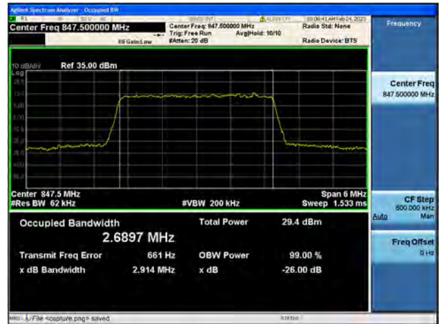
Band5 / 3MHz / QPSK/ High CH
