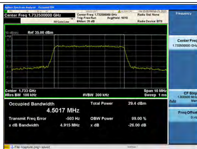
Band4 / 5MHz / 64QAM/ Mid CH
