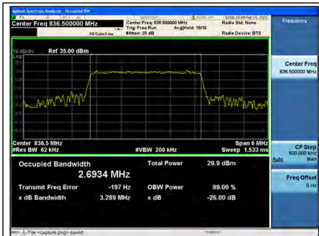
Band5 / 3MHz / QPSK/ Mid CH
