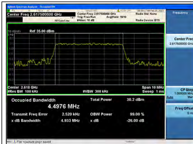
Band38 / 5MHz / QPSK/ High CH
