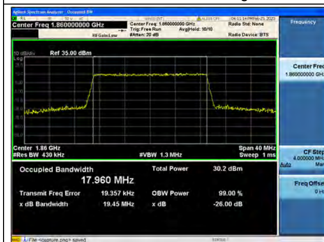
Band2 / 20MHz / 16QAM/ Low CH
