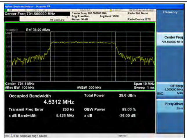
Band12 / 5MHz / 16QAM/ Low CH
