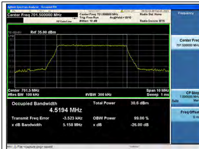
Band12 / 5MHz / QPSK/ Low CH
