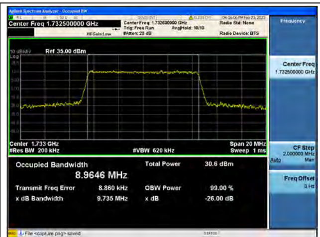
Band4 / 10MHz / 16QAM/ Mid CH
