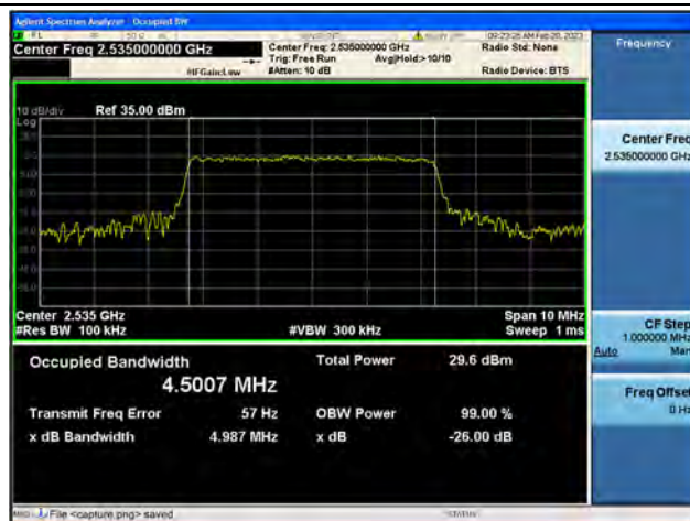
Band7 / 5MHz / 16QAM/ Mid CH
