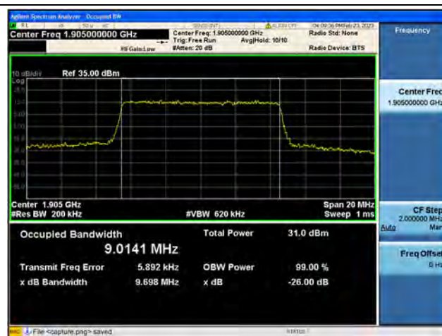
Band2 / 10MHz / QPSK/ High CH
