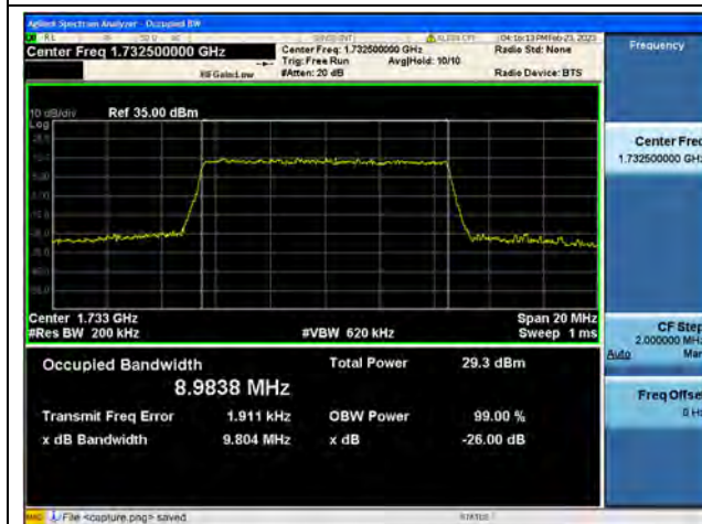
Band4 / 10MHz / 64QAM/ Mid CH
