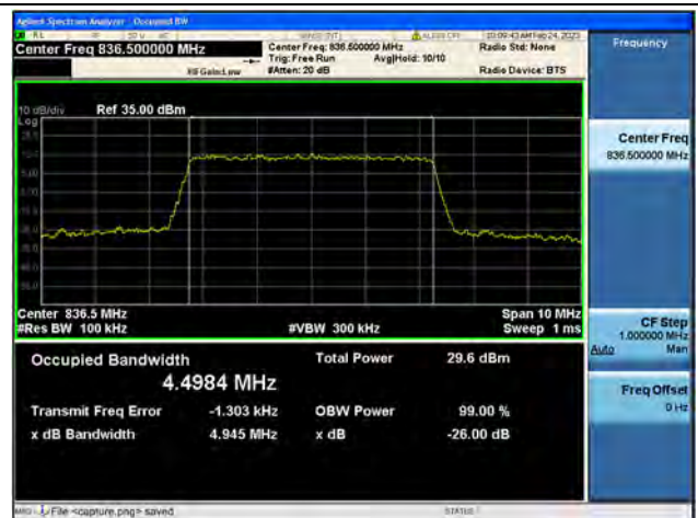
Band5 / 5MHz / 64QAM/ Mid CH
