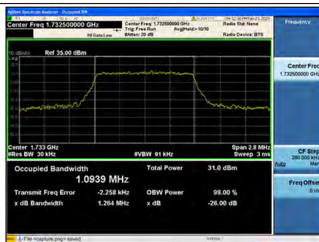
Band4 / 1.4MHz / QPSK/ Mid CH
