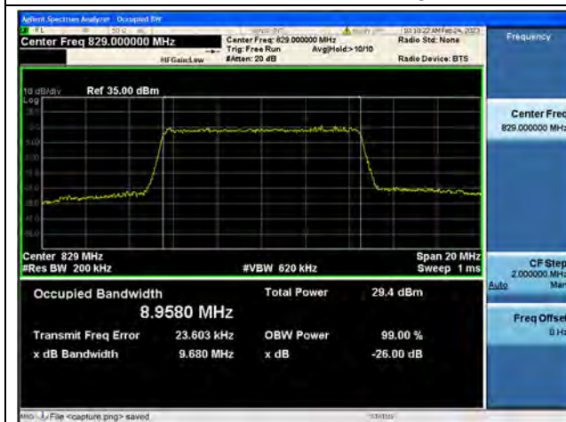
Band5 / 10MHz / 16QAM/ Low CH
