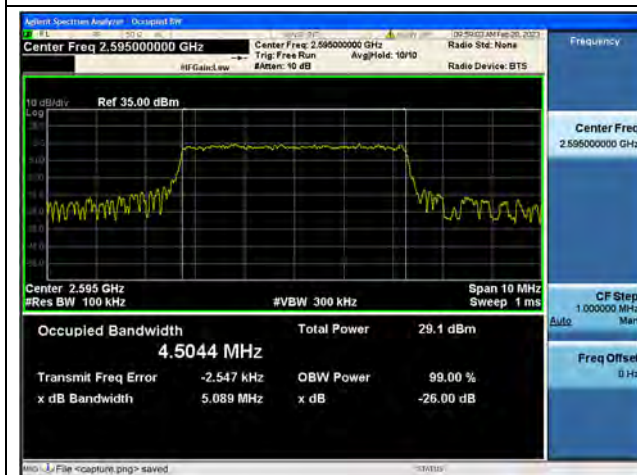
Band38 / 5MHz / 16QAM/ Mid CH
