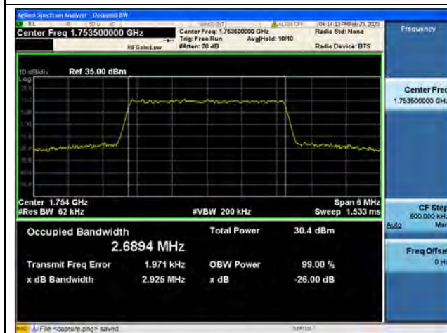
Band4 / 3MHz / 16QAM/ High CH
