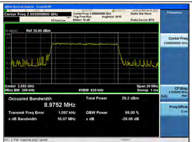
Band38 / 10MHz / 16QAM/ Mid CH
