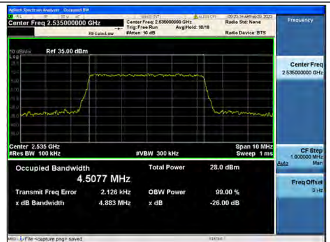
Band7 / 5MHz / 64QAM/ Mid CH
