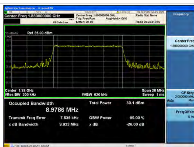
Band2 / 10MHz / 16QAM/ Mid CH
