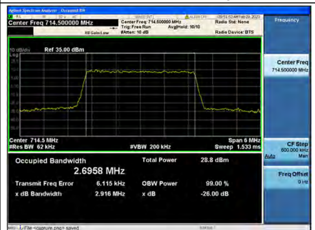
Band12 / 3MHz / 64QAM/ High CH
