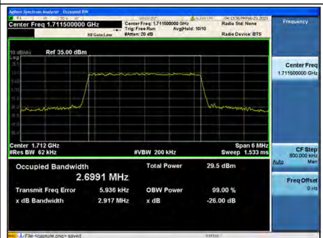
Band4 / 3MHz / 64QAM/ Low CH
