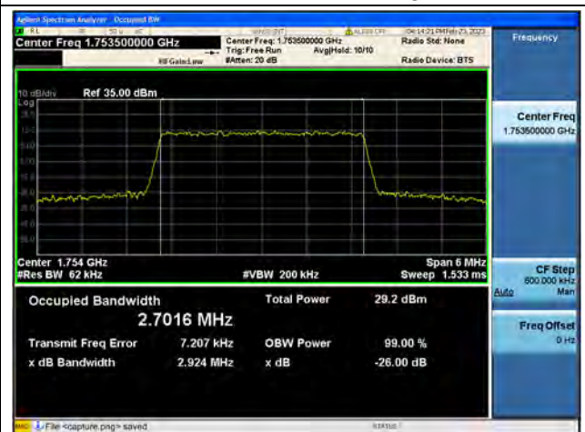
Band4 / 3MHz / 64QAM/ High CH
