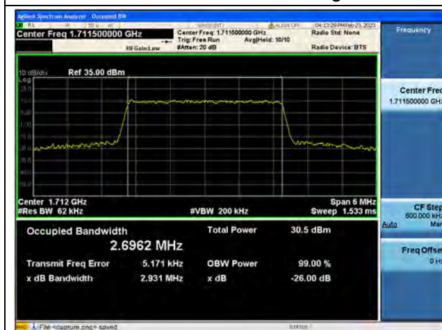
Band4 / 3MHz / 16QAM/ Low CH
