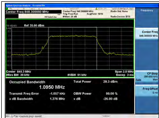
Band5 / 1.4MHz / QPSK/ High CH
