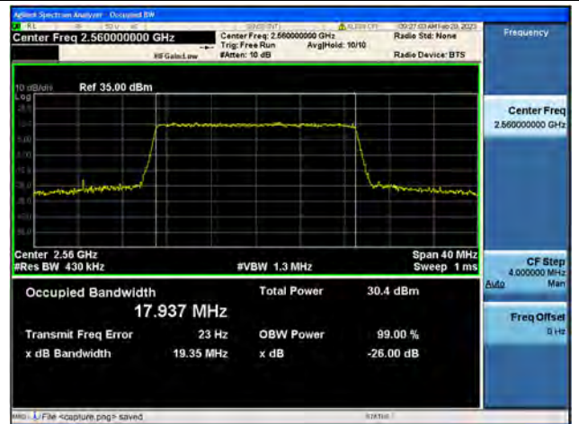
Band7 / 20MHz / QPSK/ High CH
