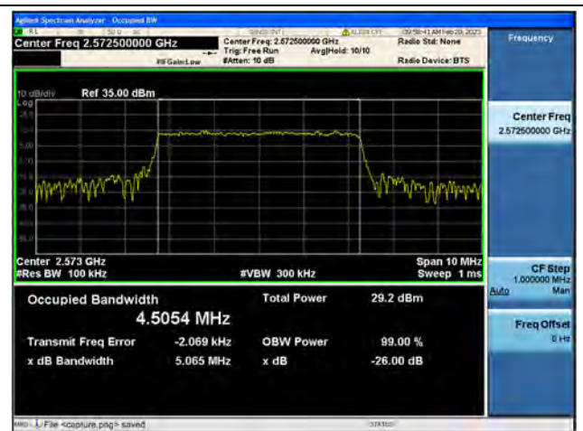
Band38 / 5MHz / 16QAM/ Low CH
