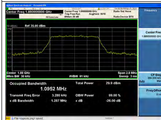
Band2 / 1.4MHz / 16QAM/ Mid CH
