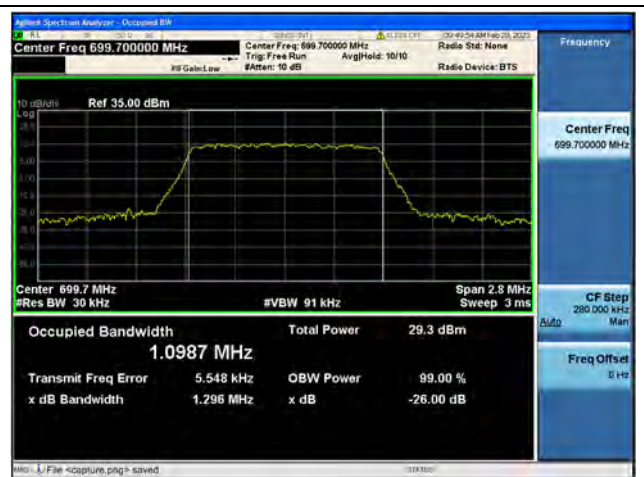
Band12 / 1.4MHz / 16QAM/ Low CH
