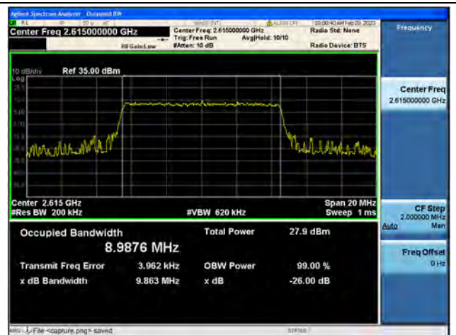
Band38 / 10MHz / 64QAM/ High CH
