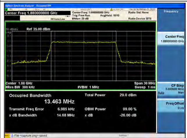
Band2 / 15MHz / 64QAM/ Mid CH
