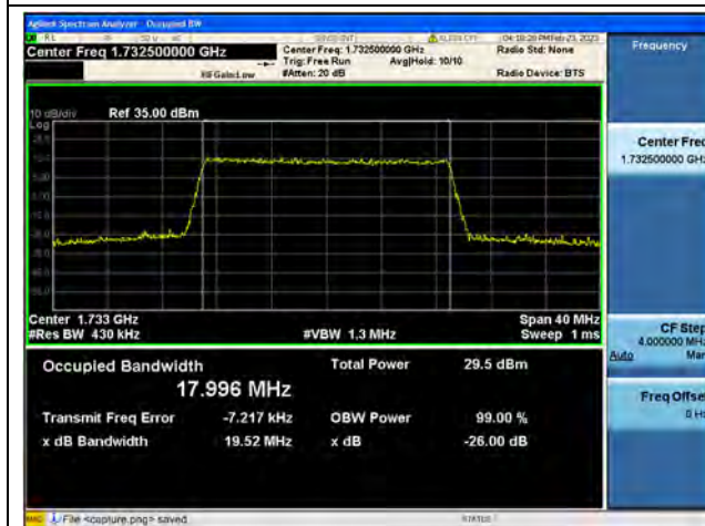
Band4 / 20MHz / 64QAM/ Mid CH
