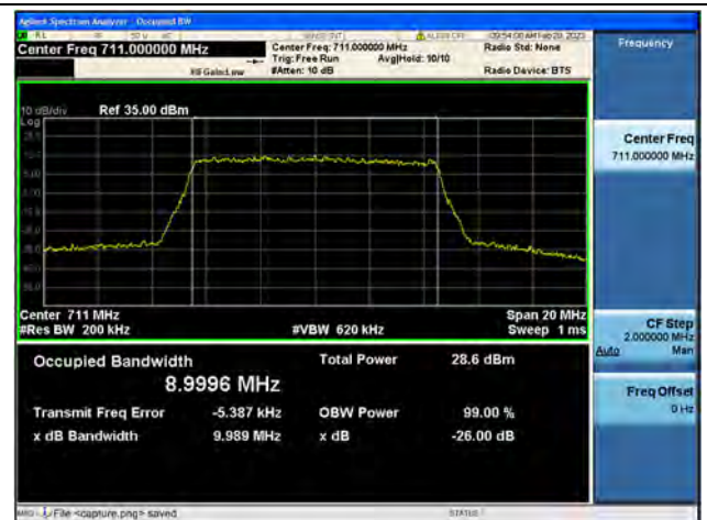
Band12 / 10MHz / 64QAM/ High CH
