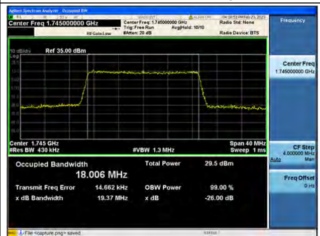
Band4 / 20MHz / 64QAM/ High CH
