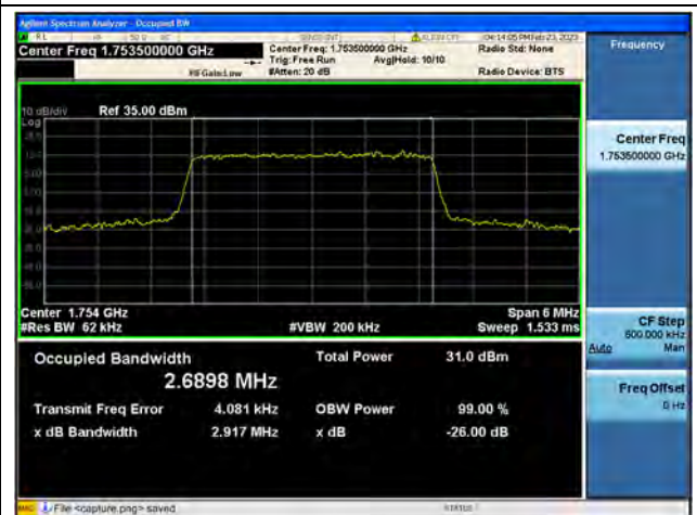
Band4 / 3MHz / QPSK/ High CH
