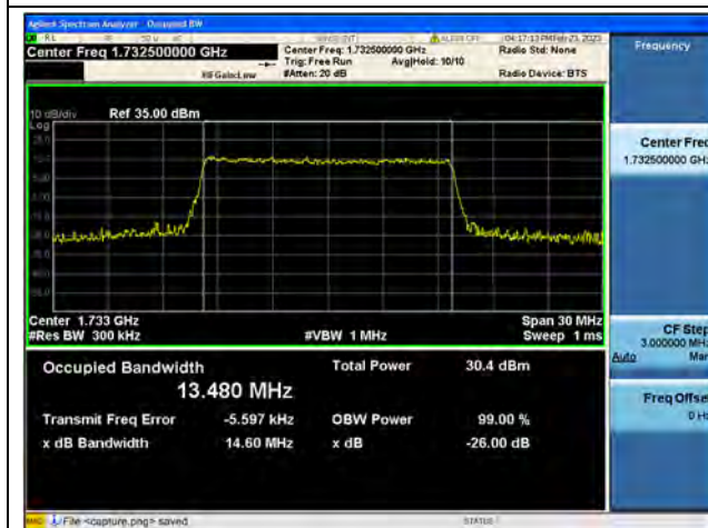
Band4 / 15MHz / 16QAM/ Mid CH
