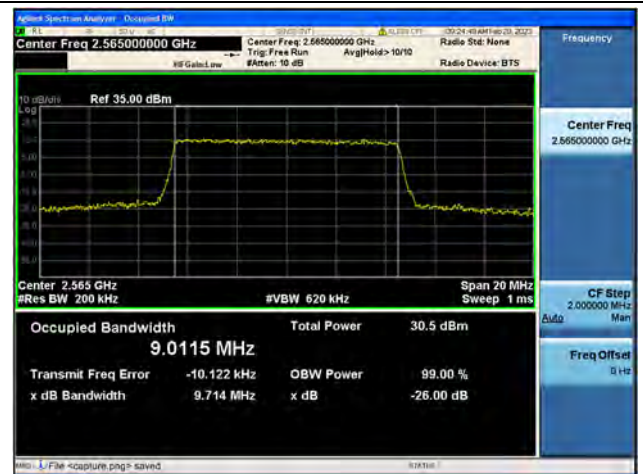
Band7 / 10MHz / QPSK/ High CH
