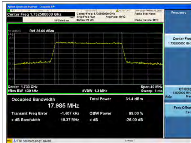
Band4 / 20MHz / QPSK/ Mid CH
