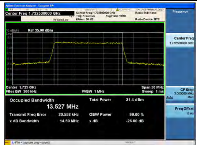
Band4 / 15MHz / QPSK/ Mid CH
