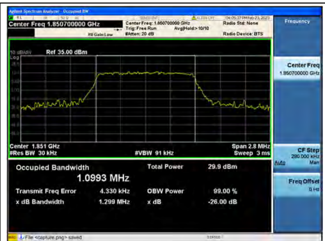
Band2 / 1.4MHz / 16QAM/ Low CH
