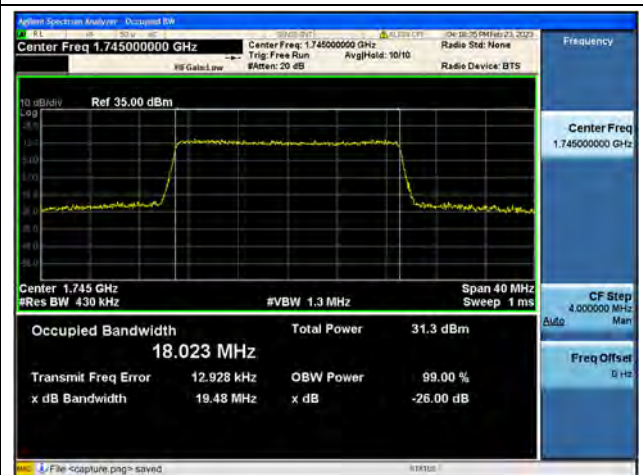
Band4 / 20MHz / QPSK/ High CH
