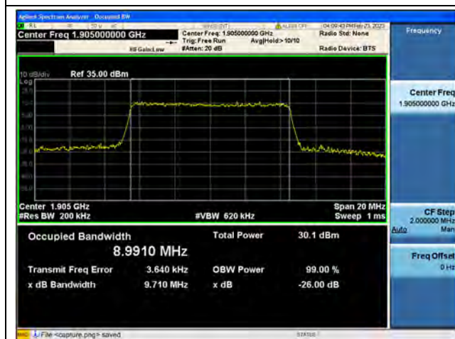
Band2 / 10MHz / 16QAM/ High CH
