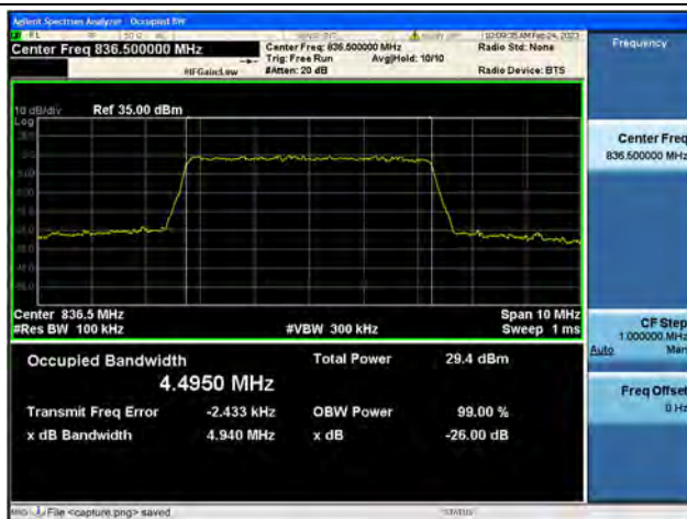
Band5 / 5MHz / 16QAM/ Mid CH
