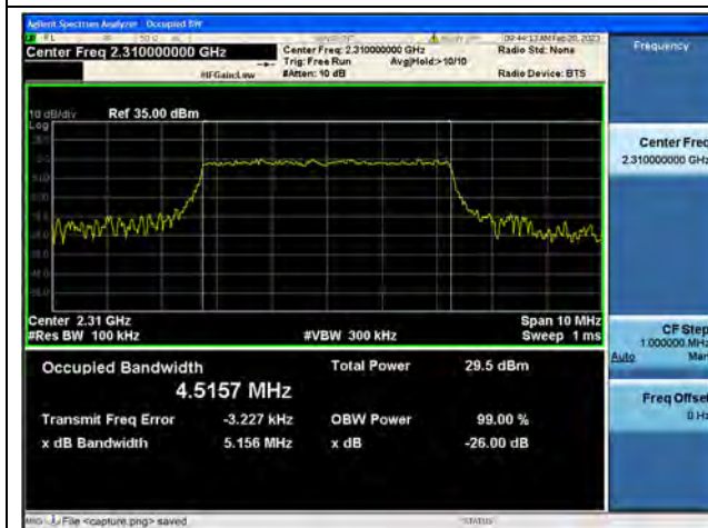
Band40-1 / 5MHz / 16QAM/ Mid CH
