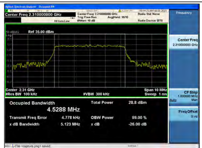
Band40-1 / 5MHz / 64QAM/ Mid CH
