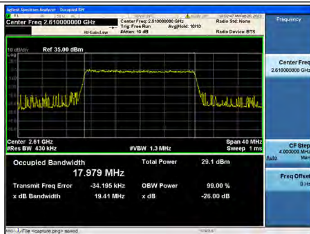
Band38 / 20MHz / 16QAM/ High CH
