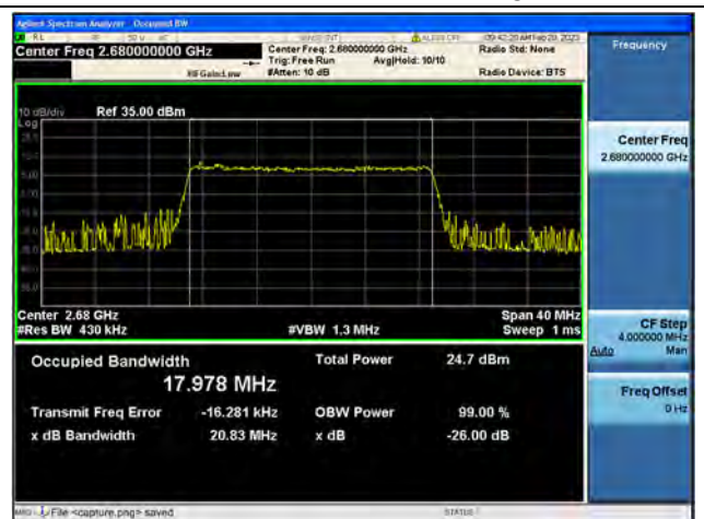
Band41 / 20MHz / 64QAM/ High CH
