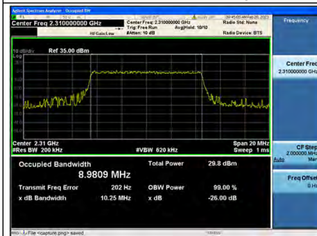
Band40-1 / 10MHz / 16QAM/ Mid CH
