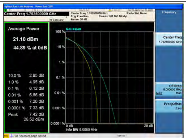
Band4 / 5MHz / High CH / 16QAM
