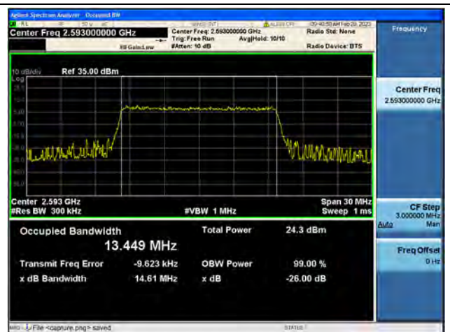
Band41 / 15MHz / 64QAM/ Mid CH
