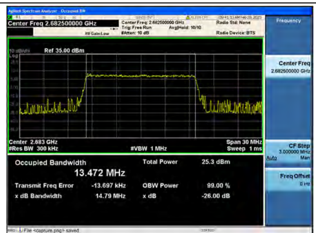
Band41 / 15MHz / 16QAM/ High CH
