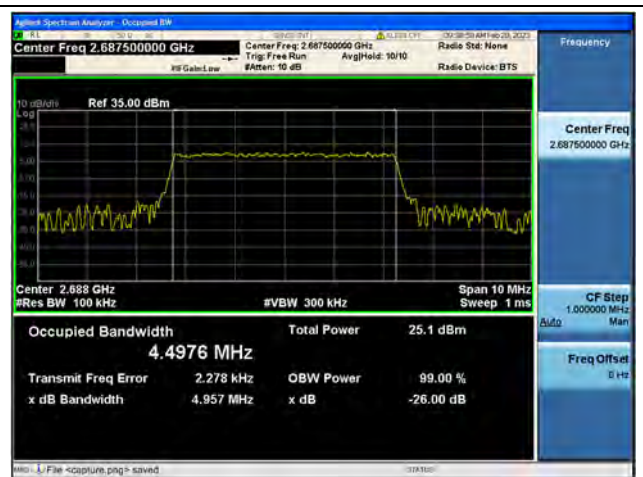
Band41 / 5MHz / 16QAM/ High CH
