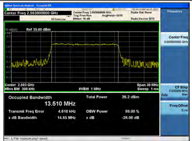
Band41 / 15MHz / QPSK/ Mid CH
