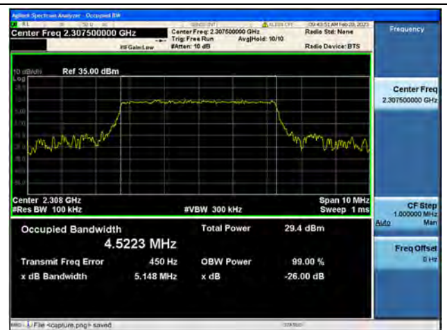
Band40-1 / 5MHz / 16QAM/ Low CH
