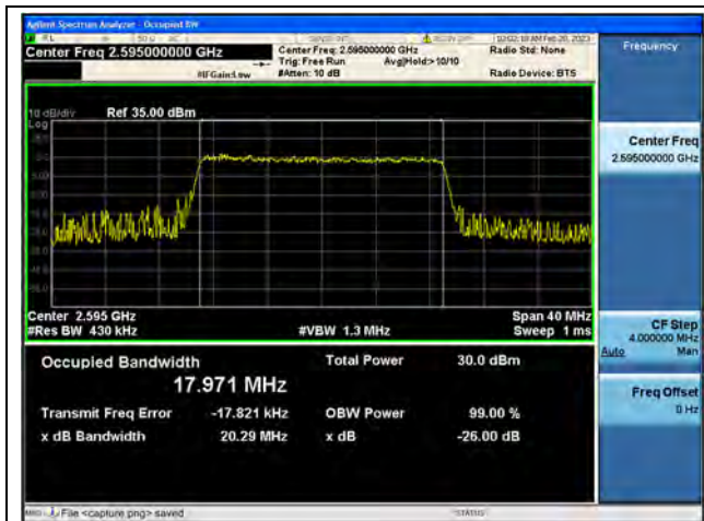
Band38 / 20MHz / QPSK/ Mid CH
