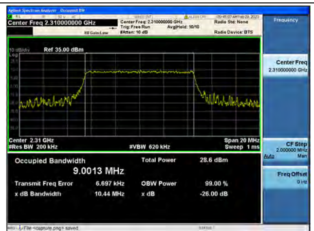
Band40-1 / 10MHz / 64QAM/ Mid CH
