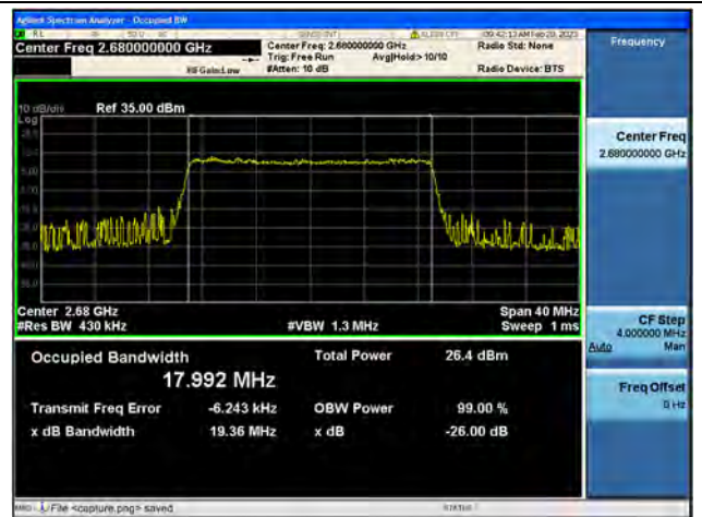
Band41 / 20MHz / QPSK/ High CH
