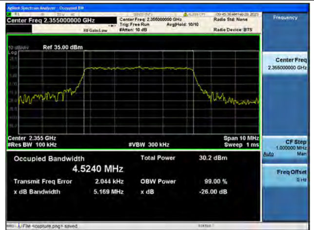
Band40-2 / 5MHz / QPSK/ Mid CH
