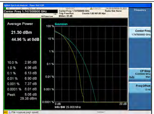
Band4 / 15MHz / High CH / 16QAM
