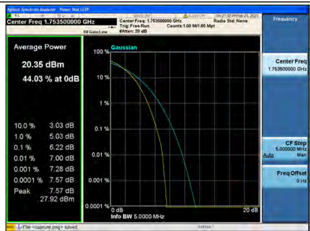
Band4 / 3MHz / High CH / 64QAM
