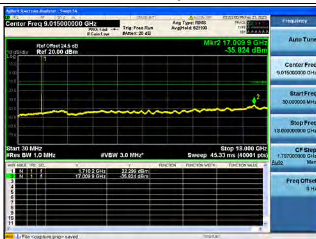
Band4 / 3MHz / Low CH / 16QAM
