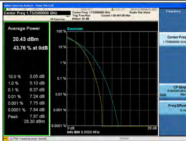
Band4 / 3MHz / Mid CH / 64QAM
