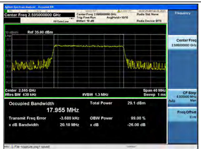
Band38 / 20MHz / 16QAM/ Mid CH
