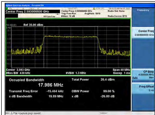
Band41 / 20MHz / QPSK/ Mid CH
