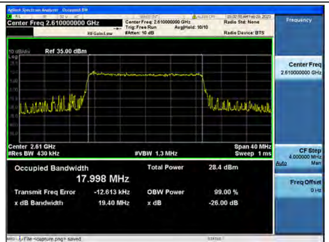
Band38 / 20MHz / 64QAM/ High CH
