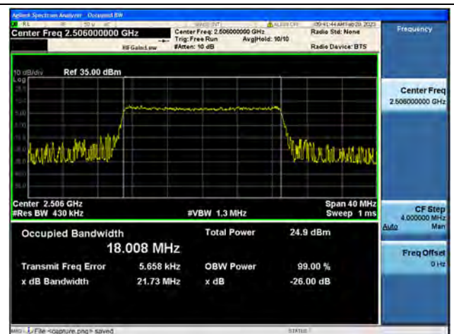
Band41 / 20MHz / 64QAM/ Low CH
