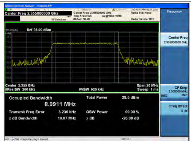
Band40-2 / 10MHz / 64QAM/ Mid CH
