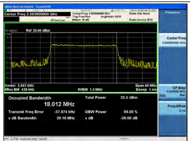
Band41 / 20MHz / 16QAM/ Mid CH
