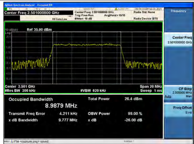
Band41 / 10MHz / QPSK/ Low CH
