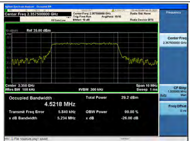
Band40-2 / 5MHz / 16QAM/ High CH
