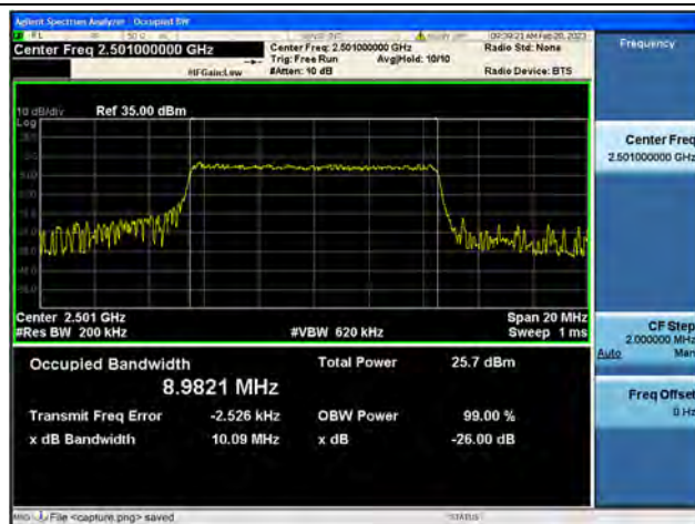
Band41 / 10MHz / 16QAM/ Low CH
