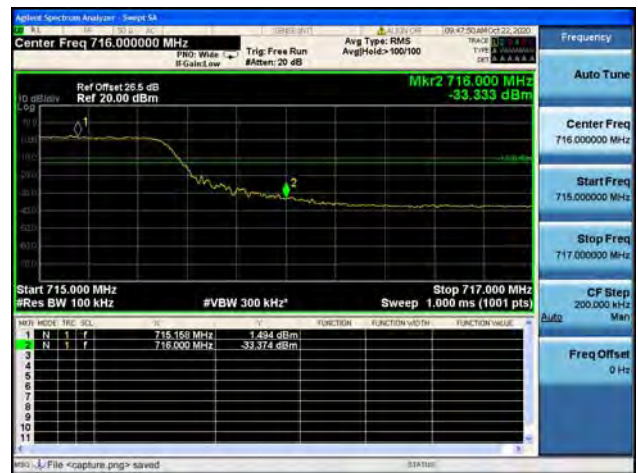
Band12 / 10MHz / High CH / QPSK / FULL RB
