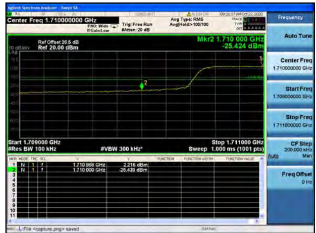
Band4 / 10MHz / High CH / QPSK / FULL RB
