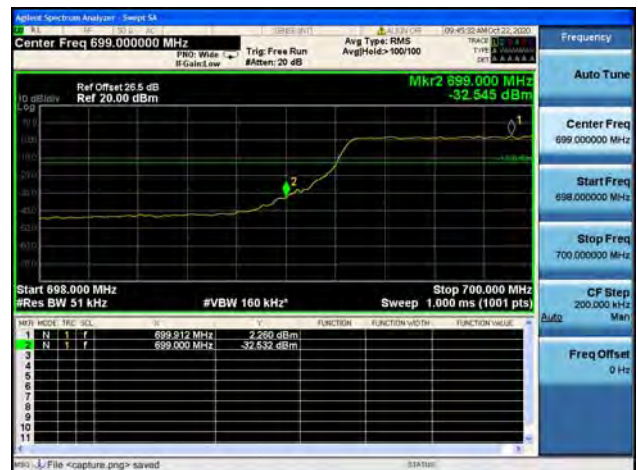
Band12 / 5MHz / High CH / QPSK / FULL RB
