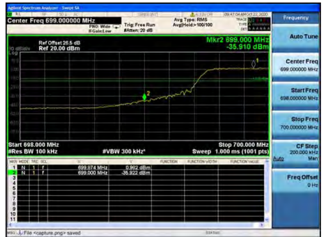
Band12 / 10MHz / High CH / QPSK / FULL RB
