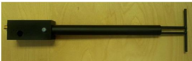
Figure 1 – MVG COMOSAR Validation Dipole
