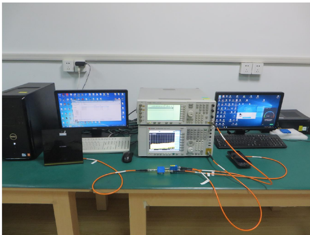
Description: DFS Test Setup
