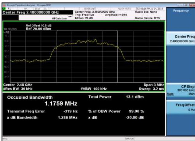
20dB Bandwidth: 8DPSK,2480MHz,3DH5
