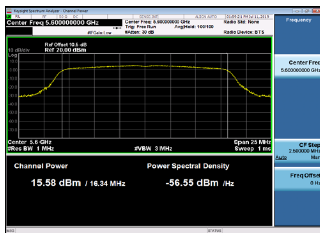
U-NII-2c Output Power-802.11a(20MHz) ,5600MHz
