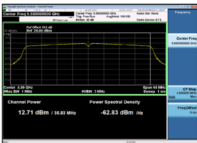
U-NII-2c Output Power-802.11a(20MHz) ,5500MHz
