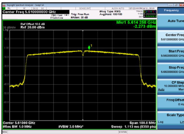
U-NII-3 Power spectral density-802.11 n(20MHz),5745MHz
