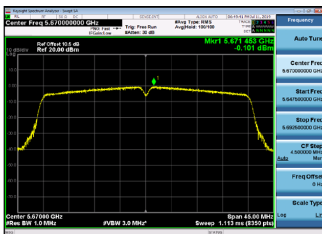
U-NII-2c Power spectral density-802.1 1a(20MHz),5600MHz
