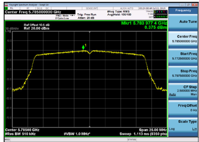
U-NII-3 Power spectral density-802.11 ac(40MHz),5755MHz
