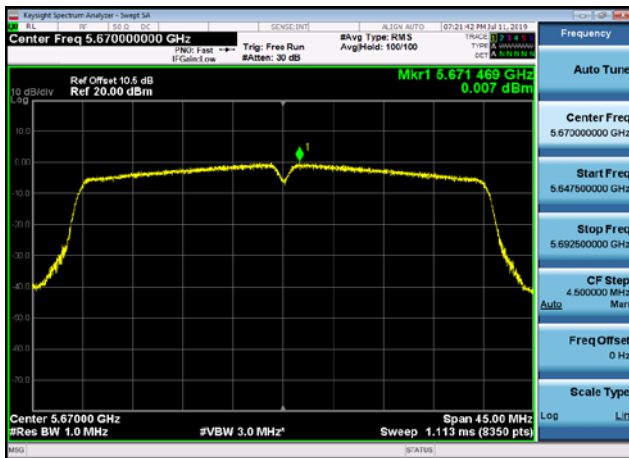
U-NII-2c Power spectral density-802.1 1ac(80MHz),5610MHz
