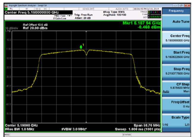
U-NII-1 Power spectral density-802.11 a(20MHz),5180MHz
