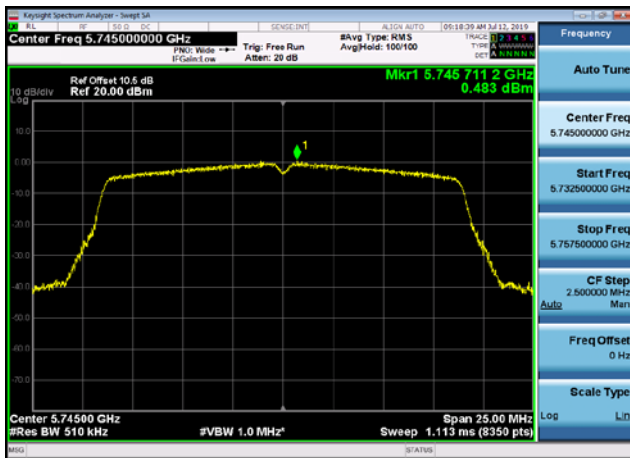
U-NII-3 Power spectral density-802.11 ac(20MHz),5825MHz
