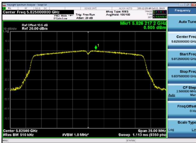
U-NII-3 Power spectral density-802.11 n(40MHz),5795MHz
