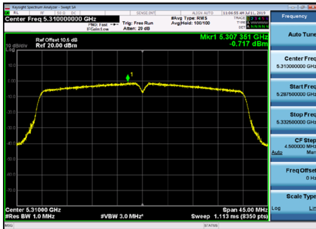
U-NII-2a Power spectral density-802.1 1ac(40MHz),5310MHz
