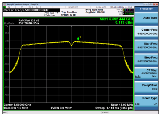
U-NII-2c Power spectral density-802.1 1a(40MHz),5590MHz
