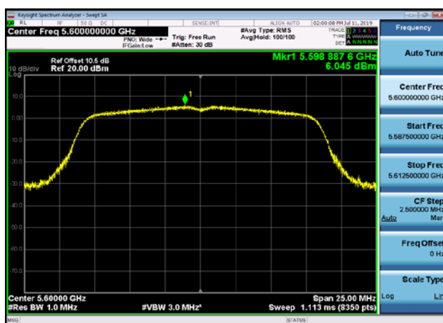
U-NII-2c Power spectral density-802.1 1a(20MHz),5600MHz
