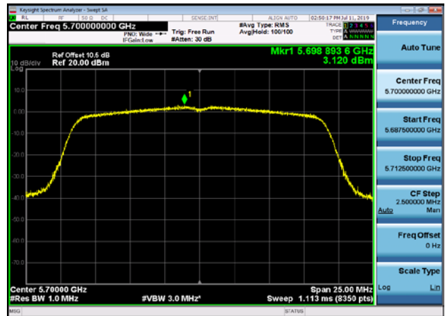
U-NII-2c Power spectral density-802.1 1a(40MHz),5590MHz
