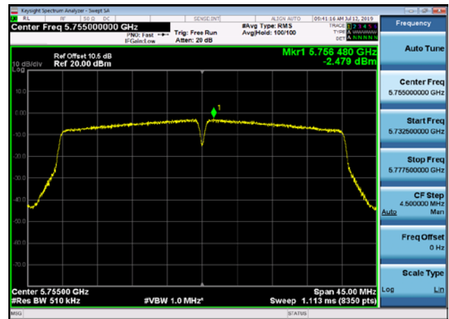
U-NII-3 Power spectral density-802.11 a(20MHz),5745MHz
