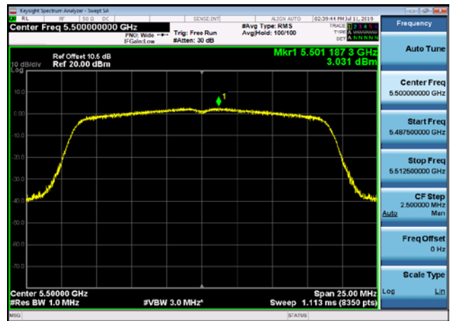
U-NII-2c Power spectral density-802.1 1a(20MHz),5700MHz
