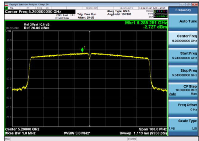
U-NII-2a Power spectral density-802.1 1ac(80MHz),5290MHz
