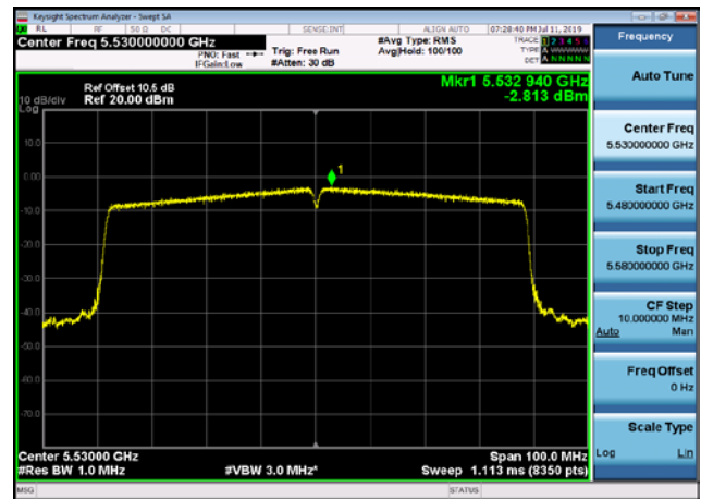
U-NII-2c Power spectral density-802.1 1ac(80MHz),5530MHz
