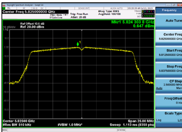
U-NII-3 Power spectral density-802.11 ac(40MHz),5795MHz
