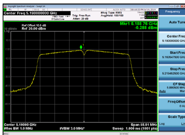
U-NII-1 Power spectral density-802.11 ac(40MHz),5190MHz
