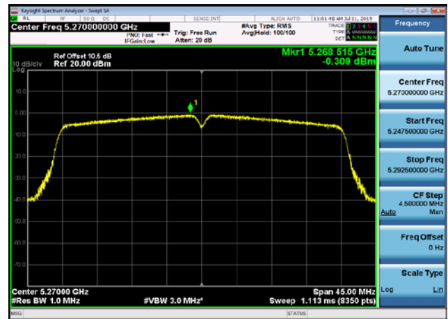
U-NII-2a Power spectral density-802.1 1ac(80MHz),5290MHz
