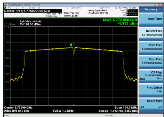
U-NII-3 Power spectral density-802.11 ac(80MHz),5775MHz
