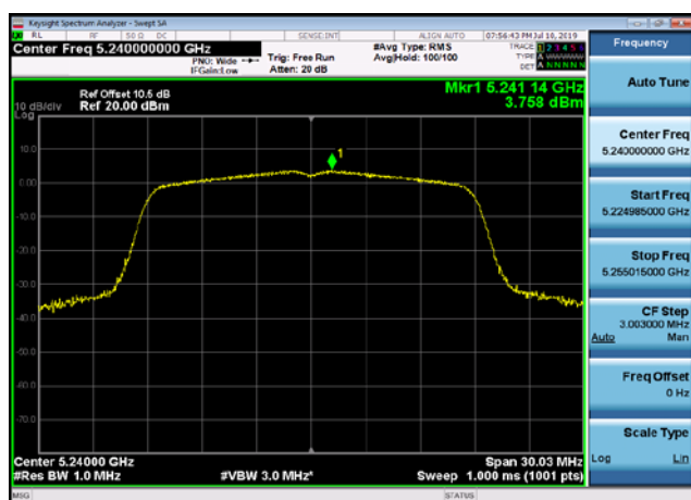
U-NII-1 Power spectral density-802.11 ac(20MHz),5240MHz
