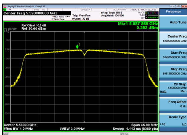
U-NII-2c Power spectral density-802.1 1a(20MHz),5500MHz
