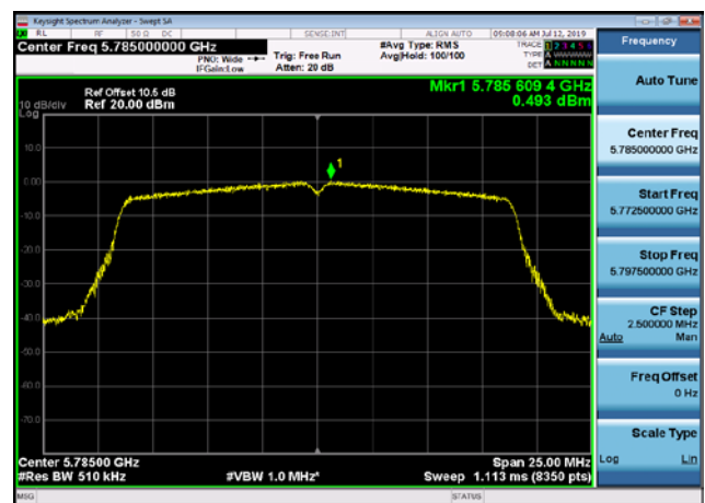
U-NII-3 Power spectral density-802.11 n(20MHz),5785MHz
