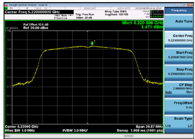
U-NII-1 Power spectral density-802.11 n(40MHz),5190MHz
