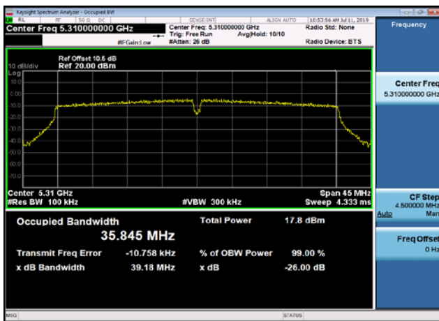
U-NII-2a 26dB Bandwidth-802.11a(20MHz ) ,5300MHz
