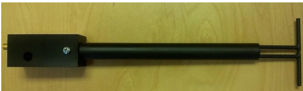
Figure 1 – MVG COMOSAR Validation Dipole
