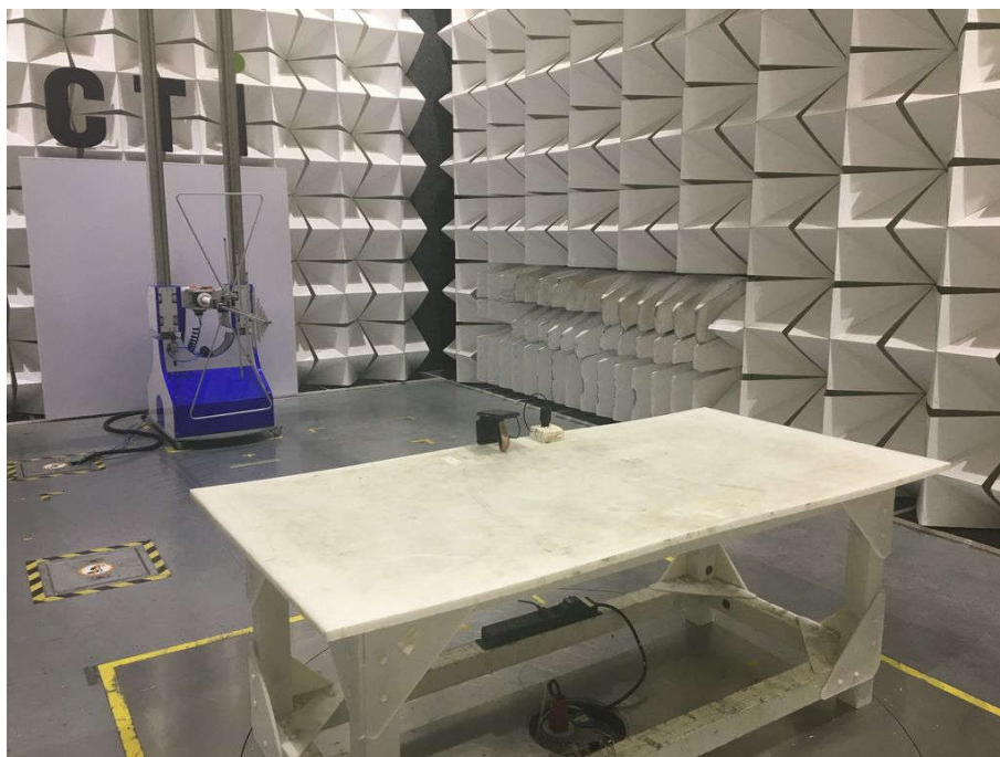
Radiated spurious emission Test Setup-1(30MHz~1GHz)
