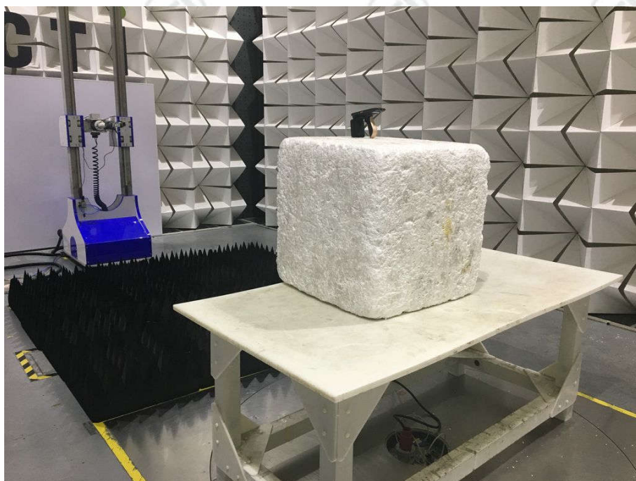
Radiated spurious emission Test Setup-3(18GHz~40GHz)
