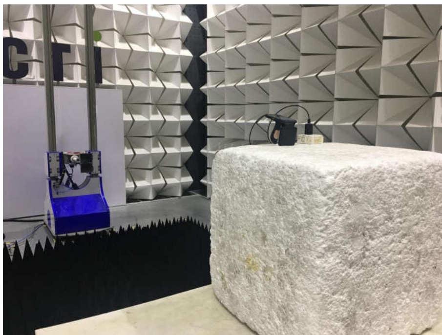
Radiated spurious emission Test Setup-2(1GHz~18GHz)
