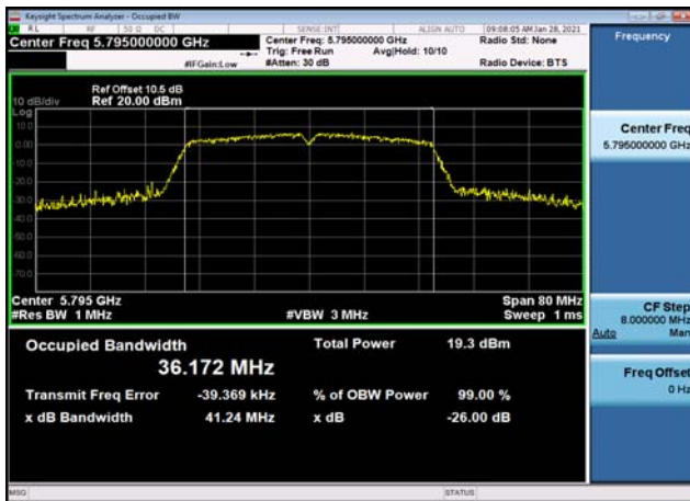
U-NII-3 99% Bandwidth-802.11a(20MHz) ,5785MHz,Ant1
