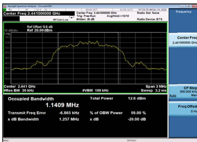
20dB Bandwidth: DQPSK,2441MHz,2DH5
