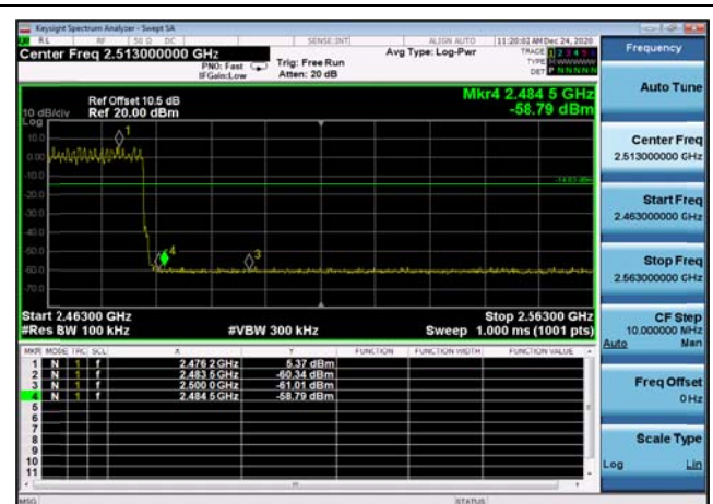
Conducted Emission: 8DPSK,2480,3DH5 ,Band Edge
