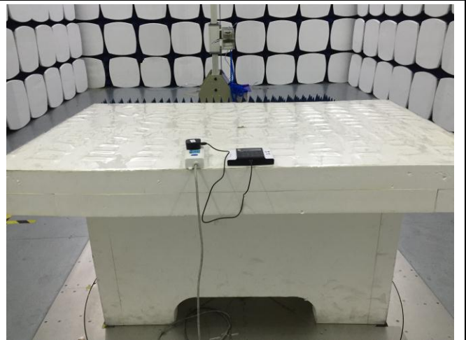
Radiated Emissions Test Setup Above 1GHz
