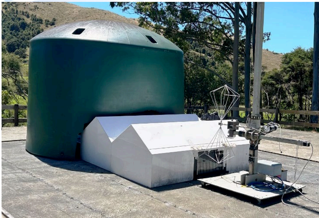
Radiated Emissions Test Site - Biconical Antenna
