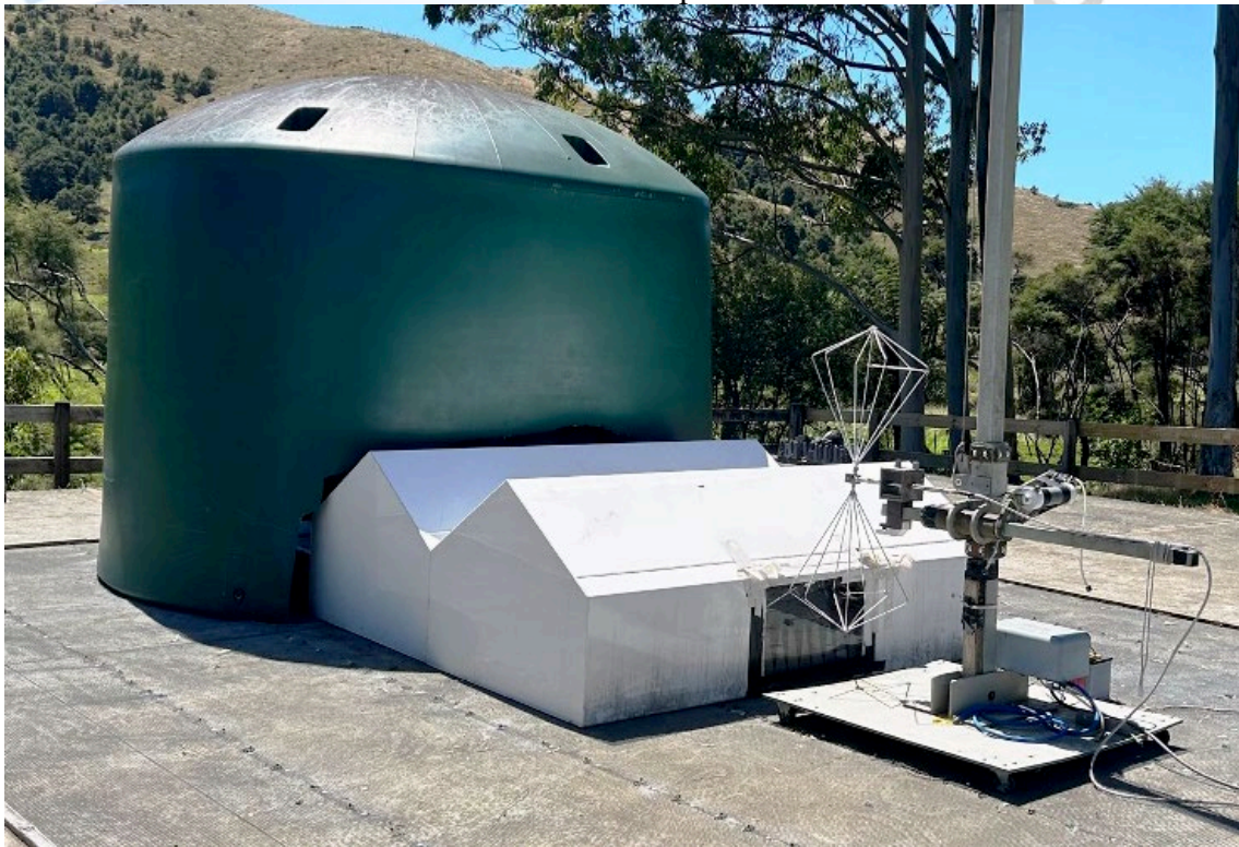
Radiated Emissions Test Setup - Biconical Antenna
