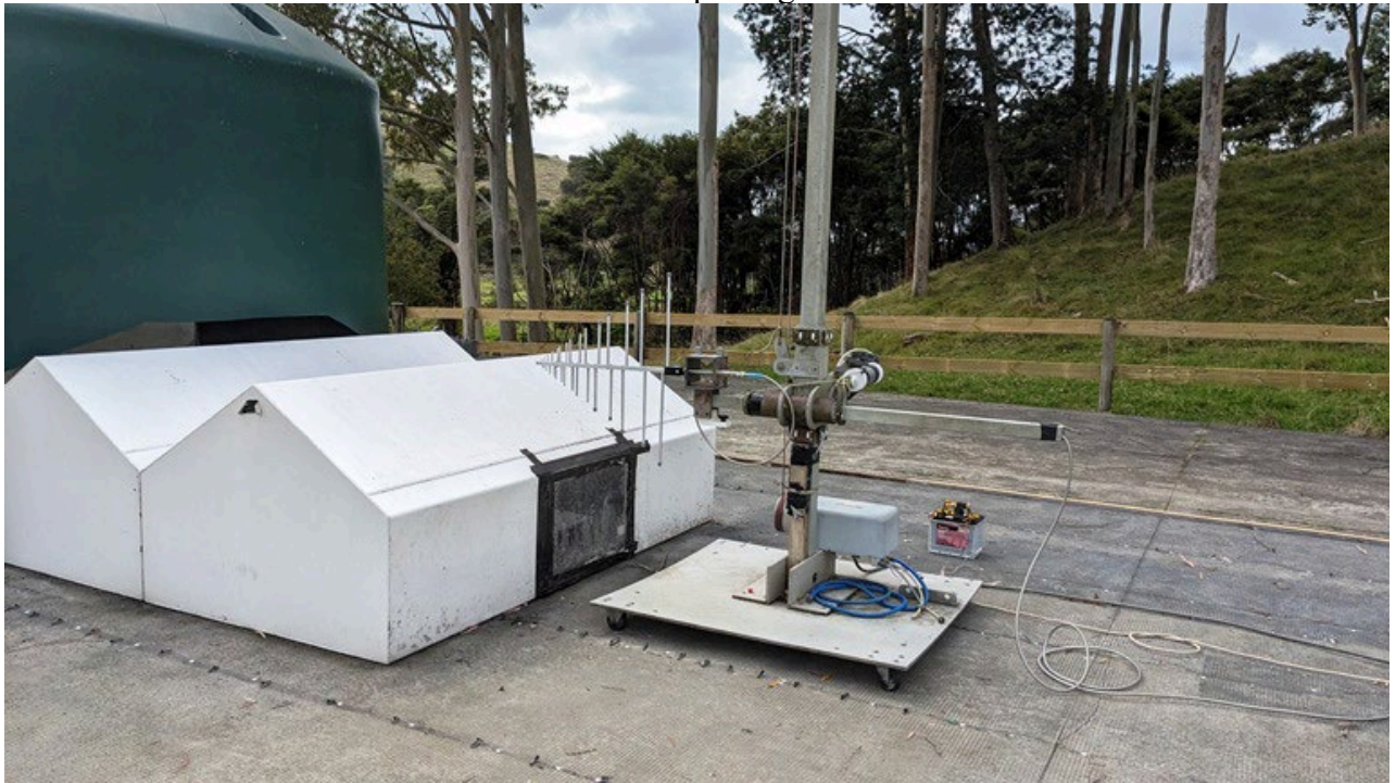
Radiated Emissions Test Setup - Horn Antenna
