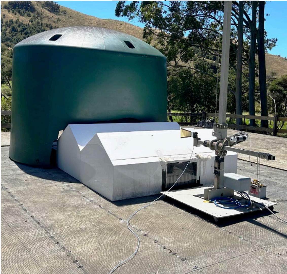
Radiated Emissions Test Setup - Horn Antenna
