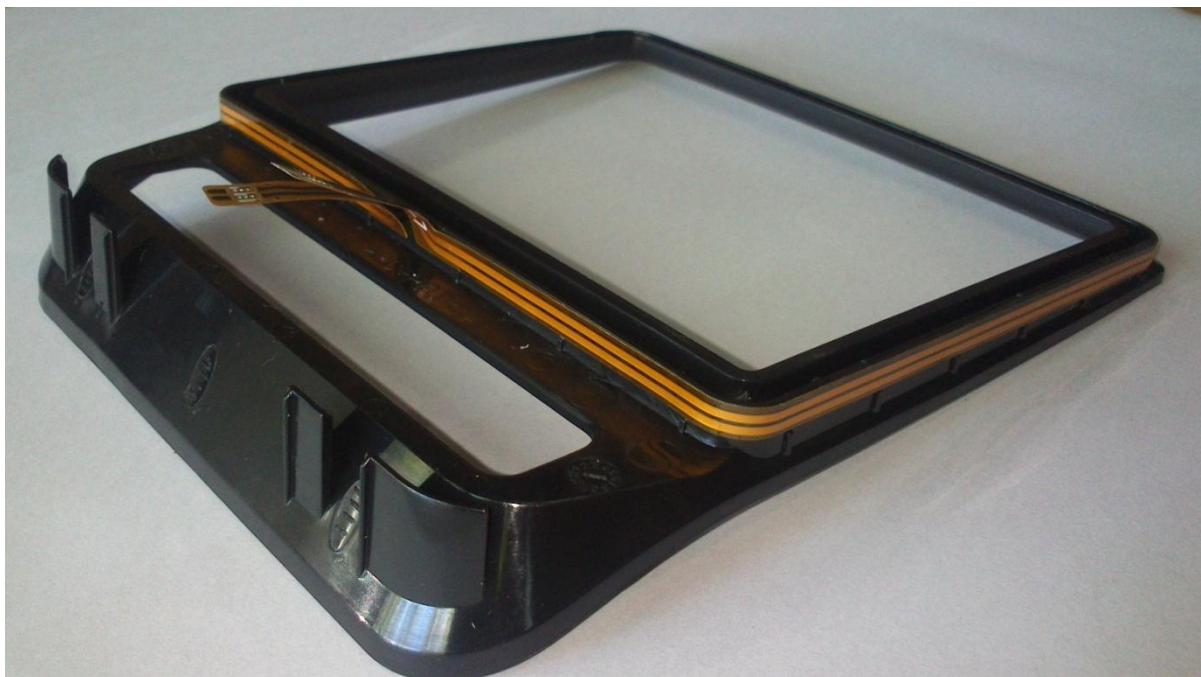
Bezel removed close up on rear side showing the contactless circuit antenna and antenna tail connection points that go to the circuit board.
