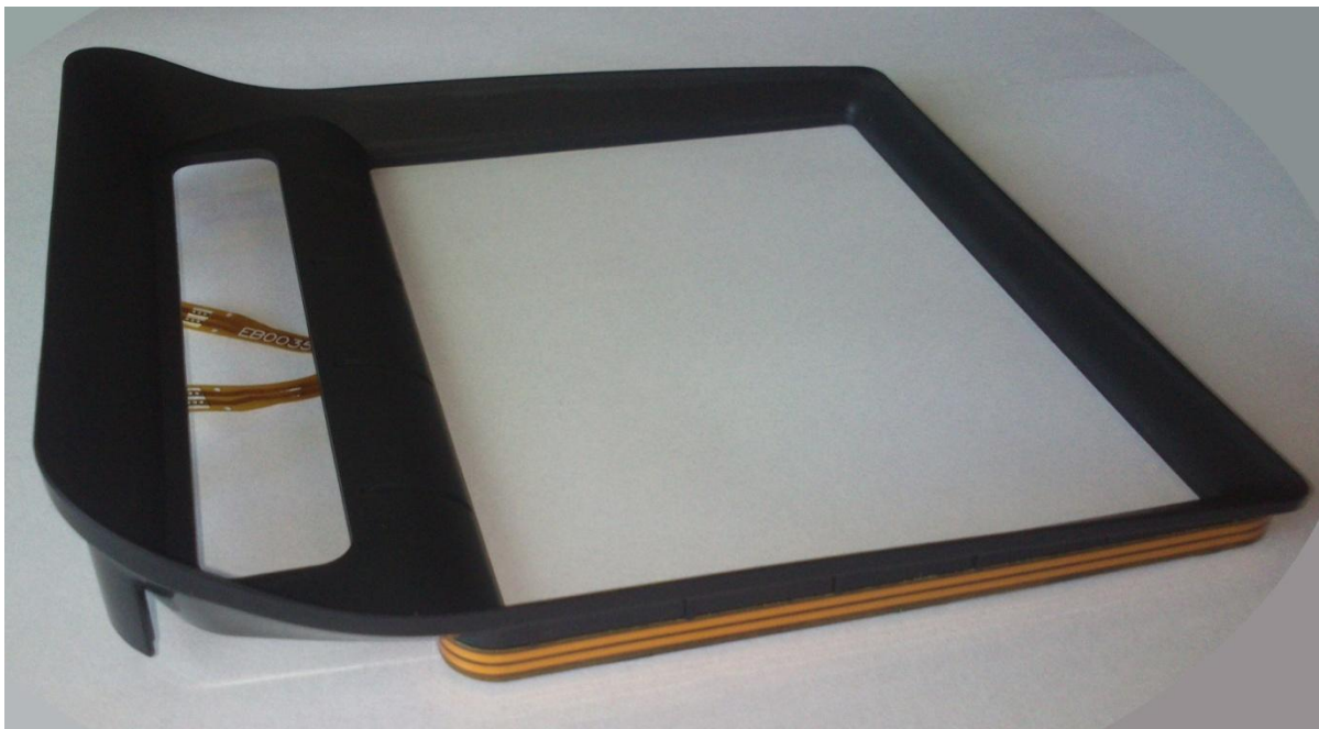
Bezel removed showing Contactless Circuit Antenna (Bezel up- Normal position).
