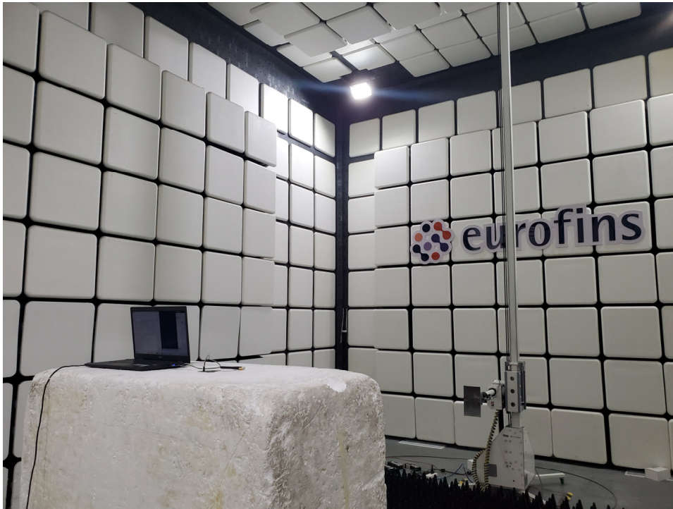
Picture 1 Radiated Emission Test Setup
