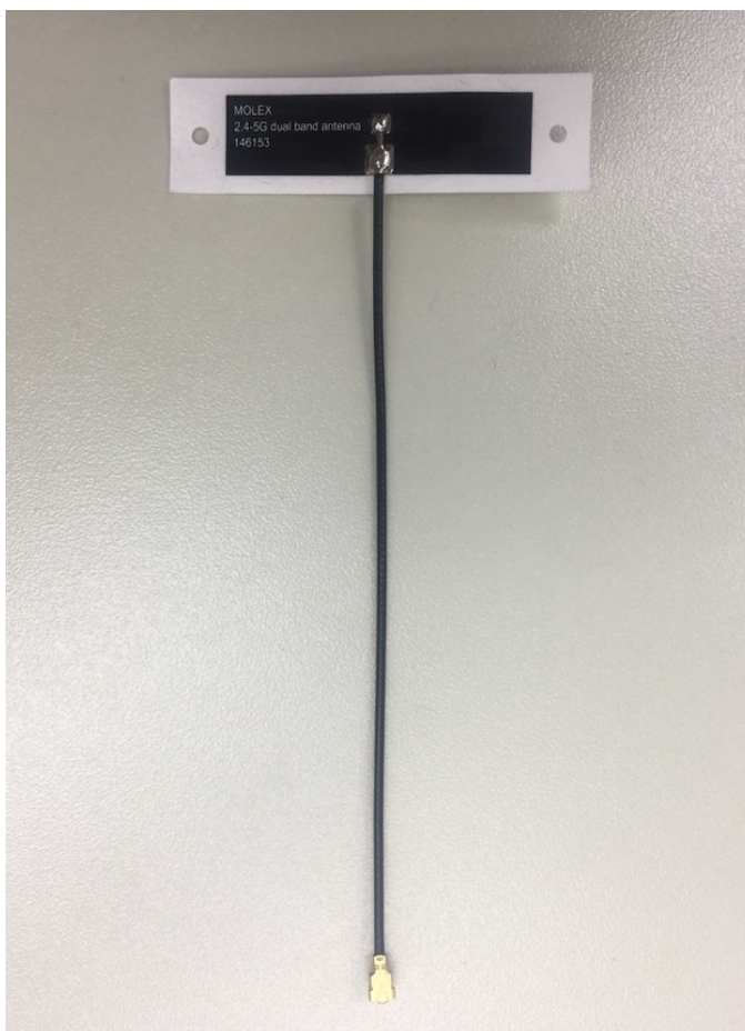
Figure 1-1. IPEX/U.FL Antenna (Top View)
