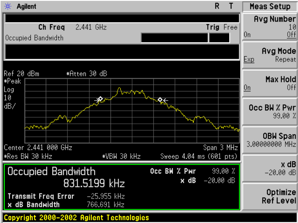
TEST PLOT OF BANDWIDTH FOR MIDDLE CHANNEL
