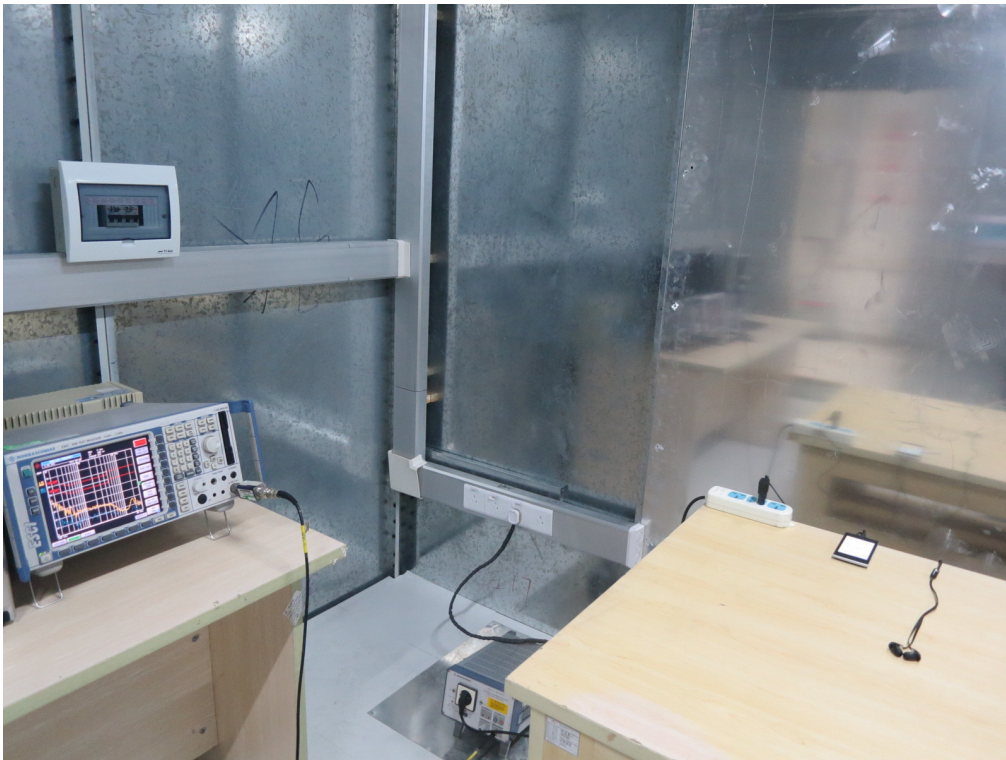
FCC LINE CONDUCTED EMISSION TEST SETUP
