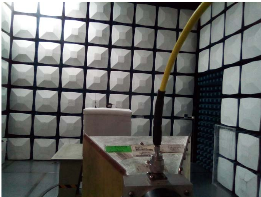
Radiated Emission View---Above 1GHz
