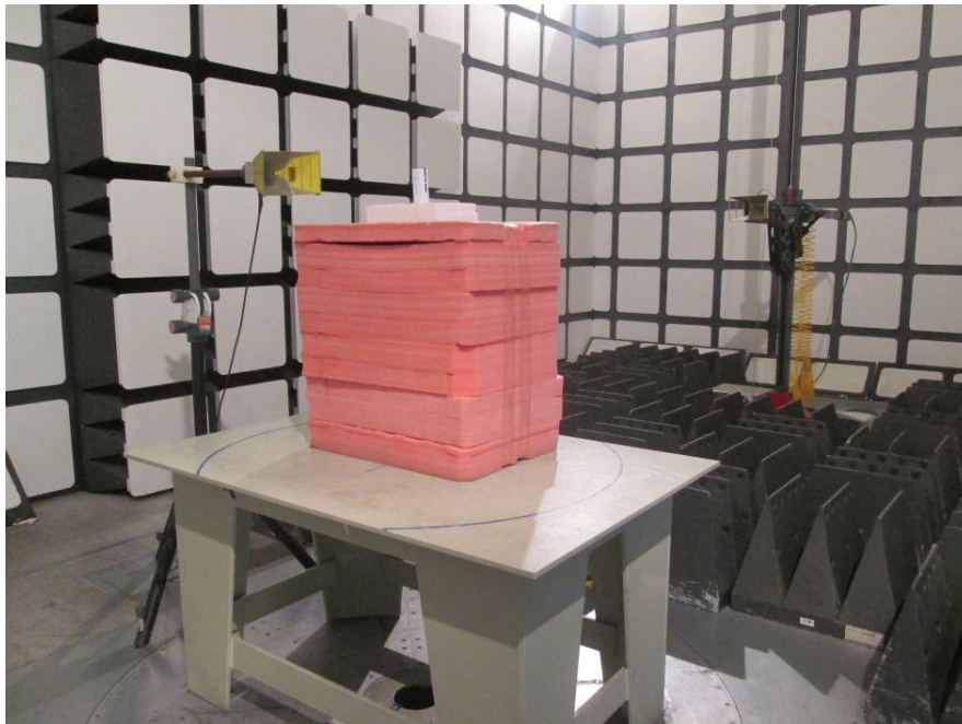
Radiated Emissions Test View (Above 1 GHz)
