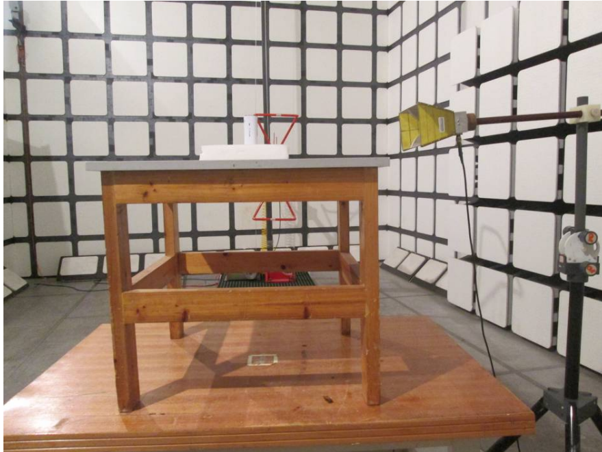
Radiated Emissions Test View (Below 1 GHz)
