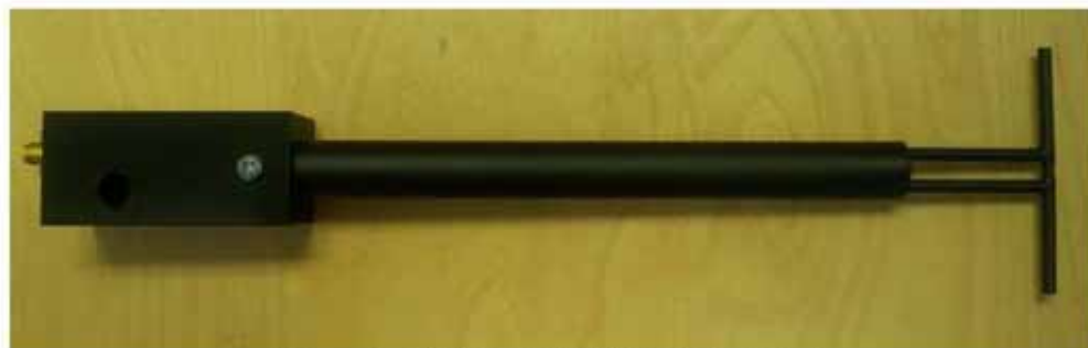
Figure 1 – MVG COMOSAR Validation Dipole
