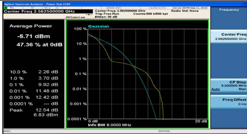
(Channel Bandwidth:15 MHz)_HCH_QPSK_1RB#37
