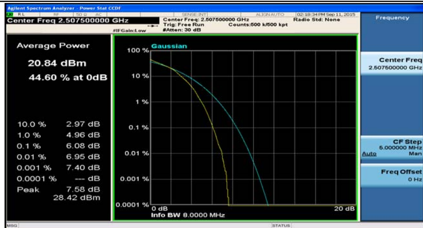
(Channel Bandwidth:15 MHz)_LCH_16QAM_37RB#38
