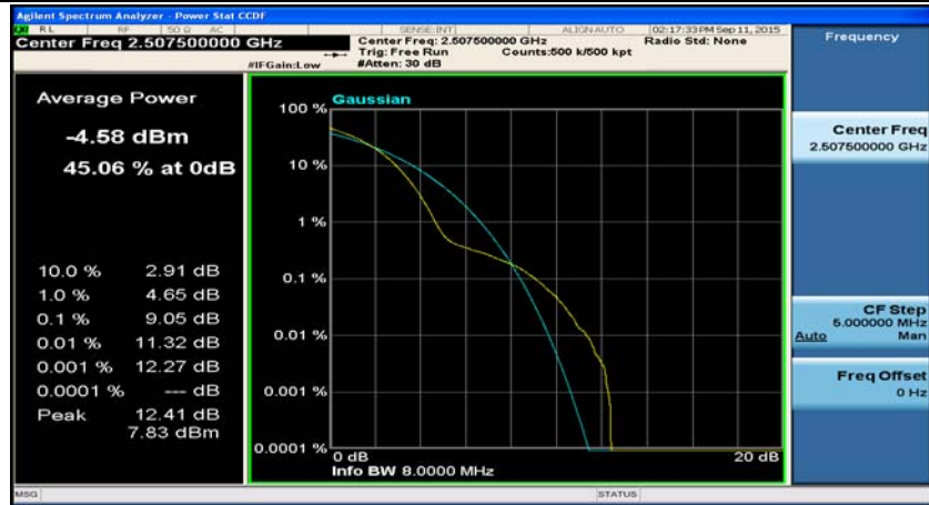
(Channel Bandwidth:15 MHz)_LCH_16QAM_37RB#0
