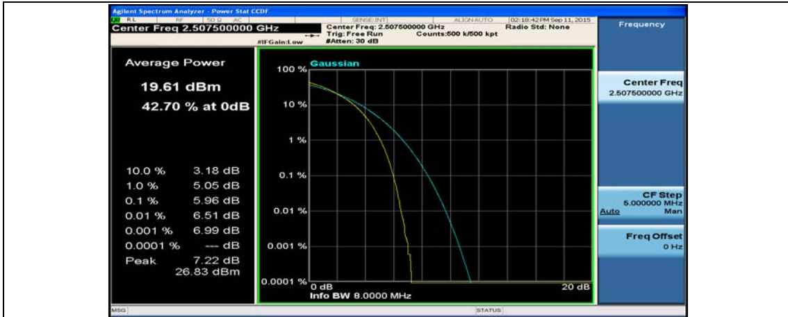
(Channel Bandwidth:15 MHz)_LCH_16QAM_75RB#0
