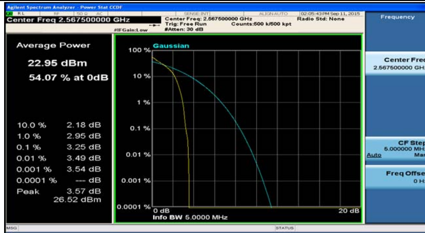
(Channel Bandwidth: 5 MHz)_HCH_QPSK_1RB#12
