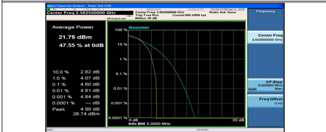
(Channel Bandwidth: 5 MHz)_LCH_16QAM_1RB#12
