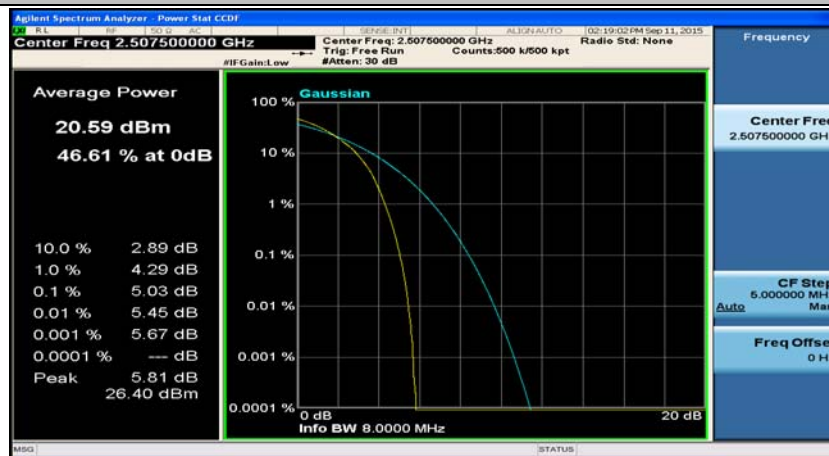
(Channel Bandwidth:15 MHz)_LCH_QPSK_75RB#0
