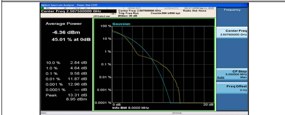
(Channel Bandwidth:15 MHz)_LCH_16QAM_1RB#37
