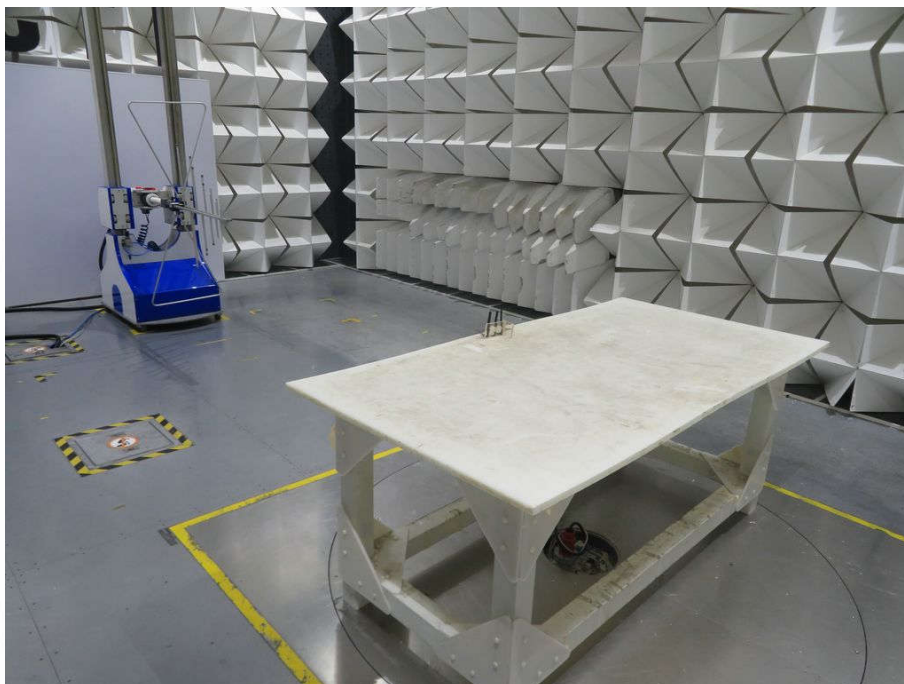
Radiated emission Test Setup-1(Below 1GHz)
