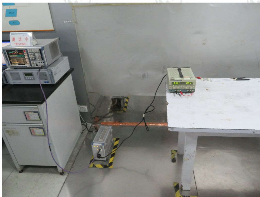
Conducted Emissions Test Setup
