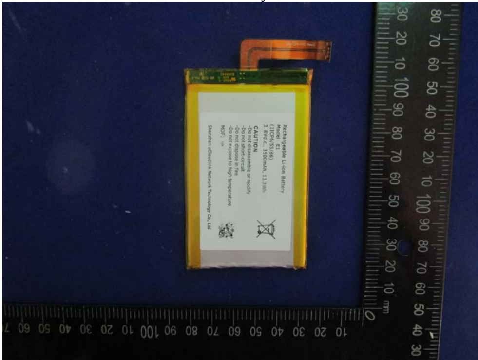
EUT – Battery View
