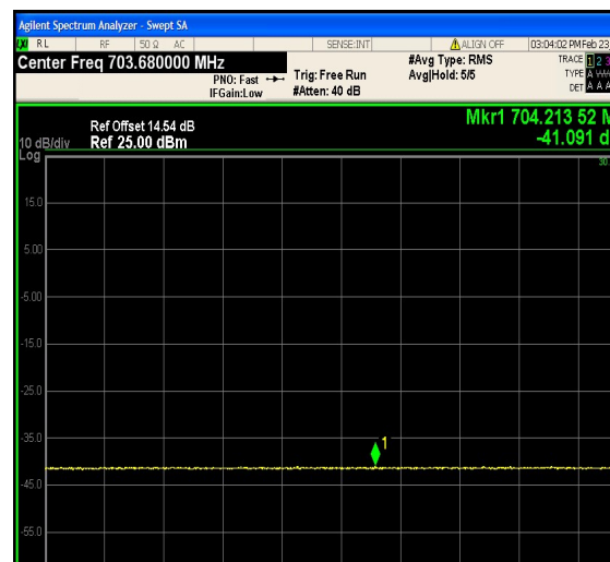
1-N12-PC3-15-10-L-6-CP-QPSK-Outer_Full- 52@0-Ant1-699.0~708.36(704.21352MHz,-4 1.09MHz,Limit30,Margin[71.09])-PASS-see graph
