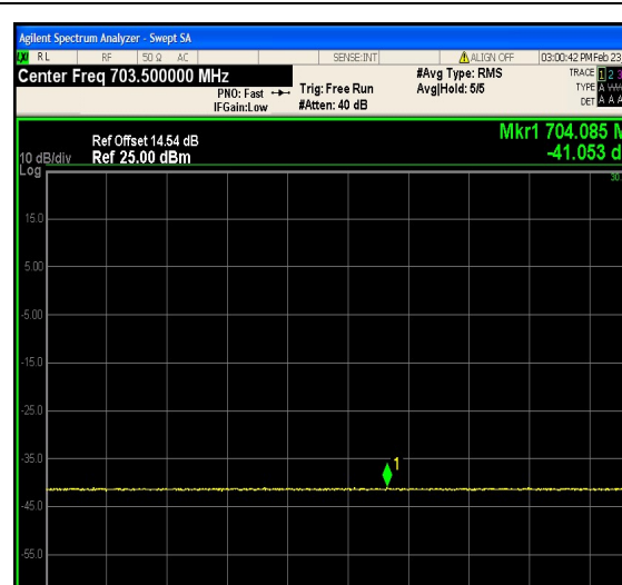
1-N12-PC3-15-10-L-3-DFT-PI2BPSK-Outer_ Full-50@0-Ant1-699.0~708.0(704.085MHz,-4 1.05MHz,Limit30,Margin[71.05])-PASS-see graph
