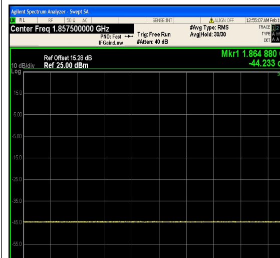
1-N25-PC3-15-15-L-4-CP-QPSK-Edge_1RB _Left-1@0-Ant1-1850.0~1865.0(1864.88MHz ,-44.23MHz,Limit30,Margin[74.23])-PASS-se e graph
