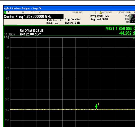
1-N25-PC3-15-15-L-3-DFT-PI2BPSK-Outer_ Full-75@0-Ant1-1850.0~1865.0(1859.885MH z,-44.26MHz,Limit30,Margin[74.26])-PASS-se e graph
