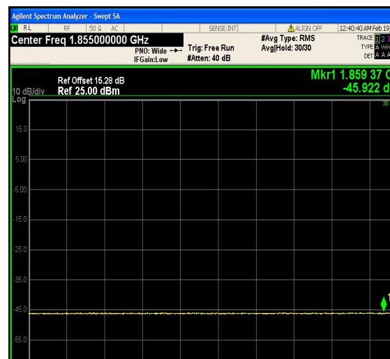
1-N25-PC3-15-10-L-6-CP-QPSK-Outer_Full- 52@0-Ant1-1850.0~1860.0(1859.37MHz,-45. 92MHz,Limit30,Margin[75.92])-PASS-see graph
