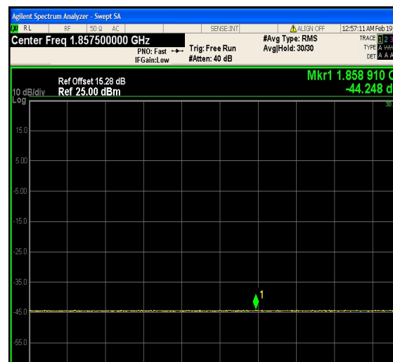
1-N25-PC3-15-15-L-6-CP-QPSK-Outer_Full- 79@0-Ant1-1850.0~1865.0(1858.91MHz,-44. 25MHz,Limit30,Margin[74.25])-PASS-see graph
