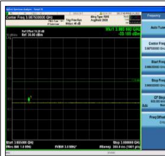
1-N77-3700-3980-PC2-30-60-H-2-DFT-PI2B PSK-Edge_1RB_Right-1@161-Ant1-3985~3 990(3985.66MHz,-33.165MHz,Limit-13,Margi n[20.165])-PASS-see graph
