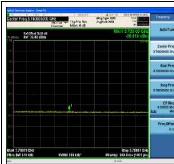
1-N77-3700-3980-PC2-30-80-L-1-DFT-PI2BP SK-Edge_1RB_Left-1@0-Ant1-3700.005~3780.005(3733.045MHz,-35.619MHz,Limit30,M argin[65.619])-PASS-see graph
