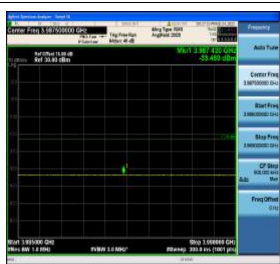
1-N77-3700-3980-PC2-30-80-H-3-DFT-PI2B PSK-Outer_Full-216@0-Ant1-3985~3990(3987.42MHz,-33.469MHz,Limit-13,Margin[20.469])-PASS-see graph
