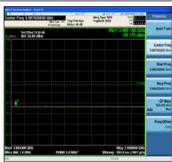
1-N77-3700-3980-PC2-30-60-H-3-DFT-PI2B PSK-Outer_Full-162@0-Ant1-3985~3990(39 85.18MHz,-33.173MHz,Limit-13,Margin[20.1 73])-PASS-see graph
