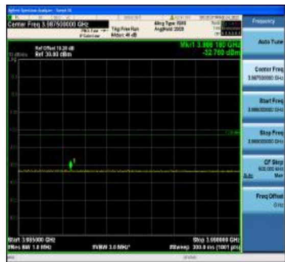
1-N77-3700-3980-PC2-30-60-H-6-CP-QPSK- Outer_Full-162@0-Ant1-3985~3990(3986.18 MHz,-32.769MHz,Limit-13,Margin[19.769])-P ASS-see graph
