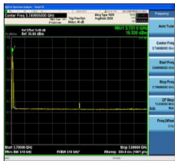
1-N77-3700-3980-PC2-30-100-L-6-CP-QPSK -Outer_Full-273@0-Ant1-3699.995~3799.995 (3700.995MHz,15.309MHz,Limit30,Margin[14 .691])-PASS-see graph
