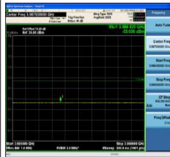
1-N77-3700-3980-PC2-30-60-H-5-CP-QPSK- Edge_1RB_Right-1@161-Ant1-3985~3990(3 986.825MHz,-33.036MHz,Limit-13,Margin[20 .036])-PASS-see graph
