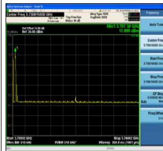
1-N77-3700-3980-PC2-30-60-L-4-CP-QPSK- Edge_1RB_Left-1@0-Ant1-3700.015~3760.015(3701.335MHz,11.966MHz,Limit30,Margin[ 18.034])-PASS-see graph
