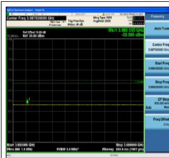
1-N77-3700-3980-PC2-30-80-H-2-DFT-PI2B PSK-Edge_1RB_Right-1@216-Ant1-3985~3990(3985.555MHz,-33.385MHz,Limit-13,Margin[20.385])-PASS-see graph
