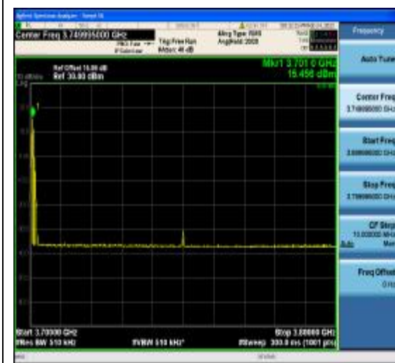
1-N77-3700-3980-PC2-30-100-L-4-CP-QPSK -Edge_1RB_Left-1@0-Ant1-3699.995~3799. 995(3700.995MHz,15.456MHz,Limit30,Margi n[14.544])-PASS-see graph
