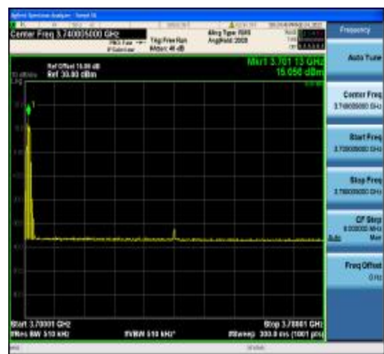
1-N77-3700-3980-PC2-30-80-L-6-CP-QPSK- Outer_Full-217@0-Ant1-3700.005~3780.005(3701.125MHz,15.056MHz,Limit30,Margin[14. 944])-PASS-see graph
